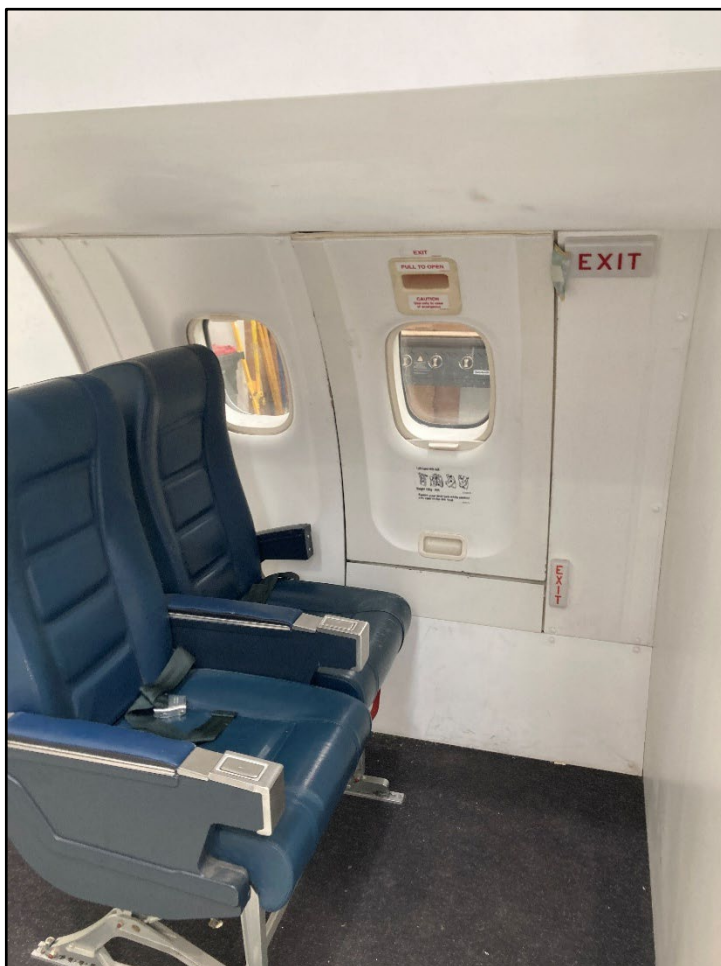
Figure 15: Type III exit installed in cabin trainer
