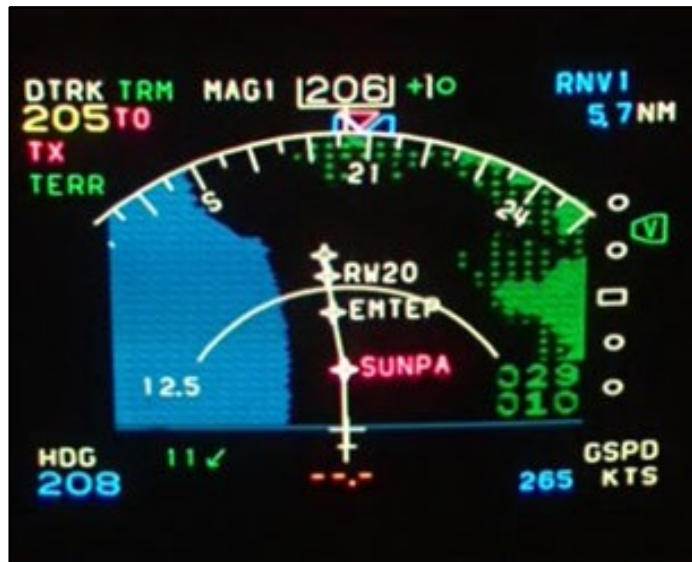
Figure 9: EHSI displaying the aeroplane has 5.7 NM to run until waypoint SUNPA
