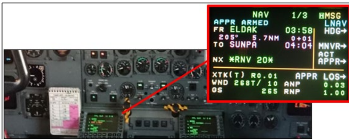
Figure 10: MCDU showing the aeroplane has 5.7 NM to run until waypoint SUNPA
