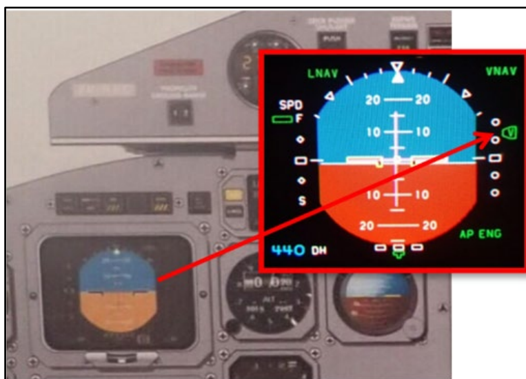
Figure 7: Flight director indicating FMS is in VNAV mode and below profile ('fly up')
