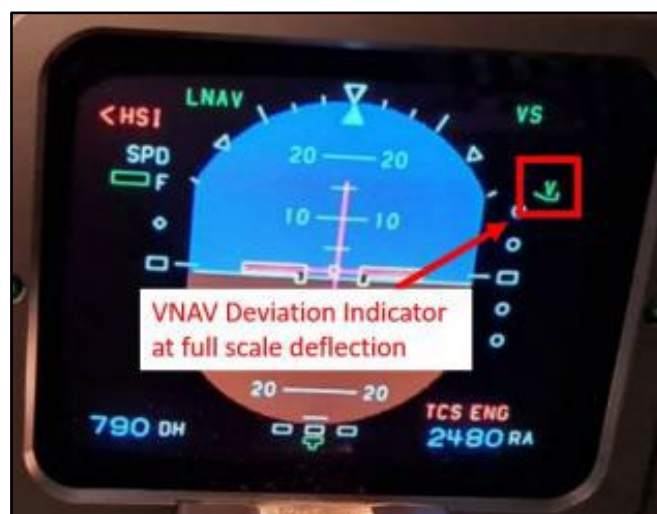
Figure 8: FMS is in V/S mode and vertical deviation annunciator is at full deflection
