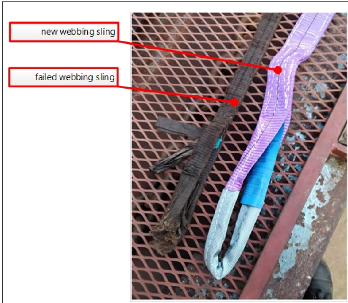
Figure 8: Comparison of the failed web sling and a new similar web sling
