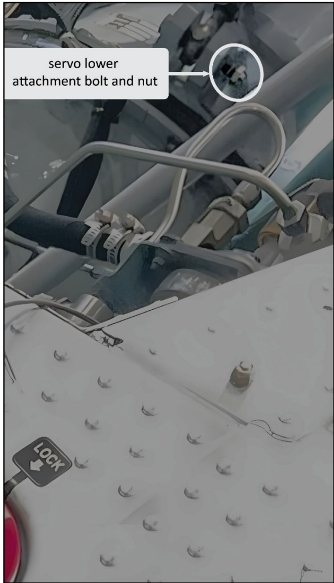
Figure 7: ZK-HJM lower attachment bolt and nut during maintenance (Credit: Engineer A, marked up by TAIC)
