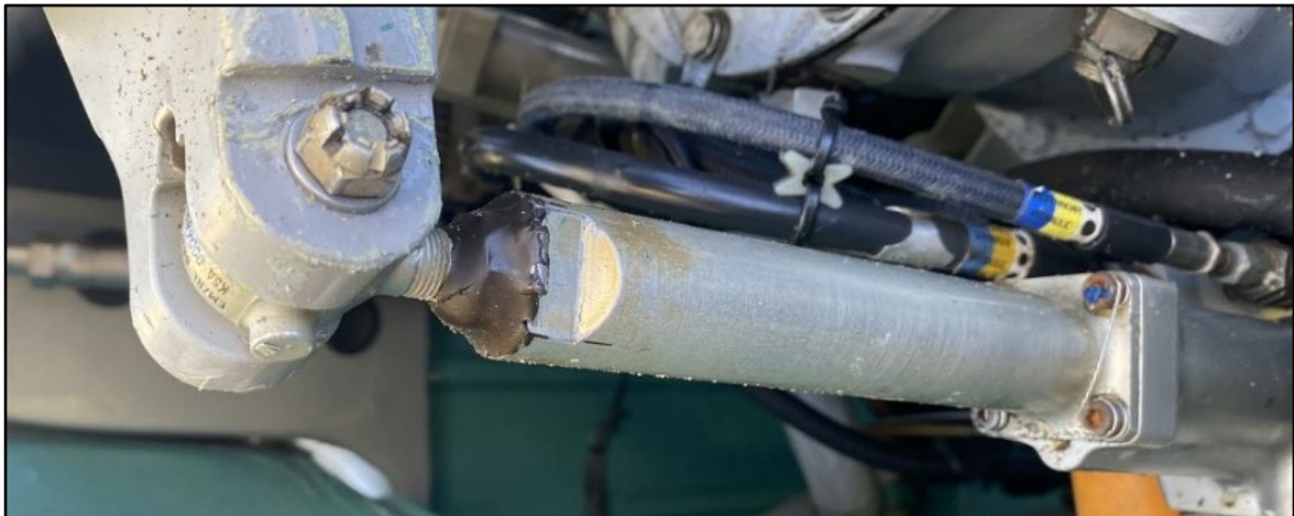
Figure 8: Left hydraulic servo upper attachment point, taken post-accident (Credit: TAIC)
