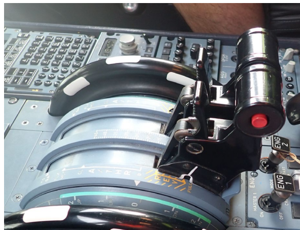
Figure 14: Thrust lever and reverser tab positions
