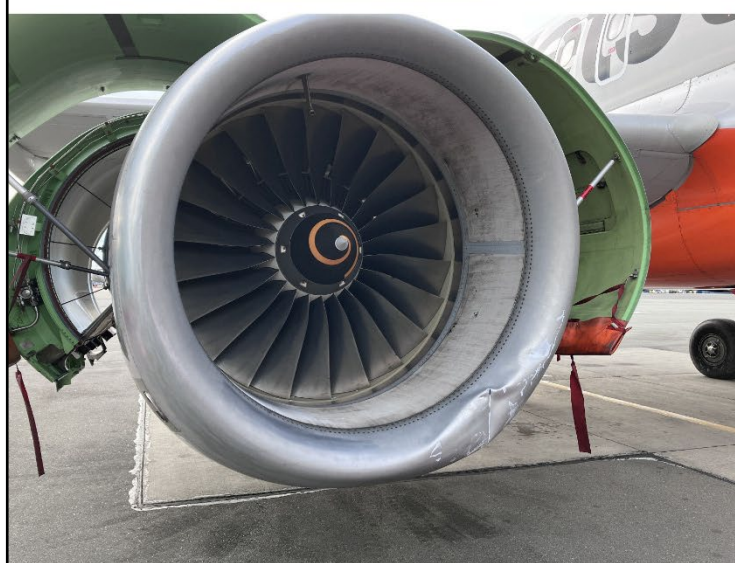
Figure 7: Engine damage from MAGS sign impact
