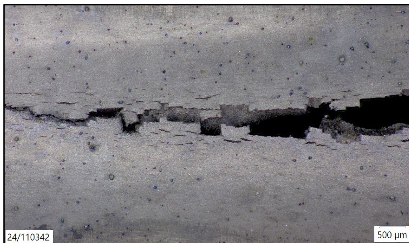
Figure 11: Inside surface stress cracks
