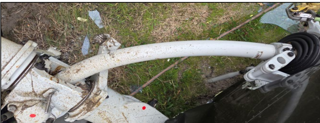
Figure 6: Main rotor mast bend
