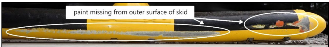
Figure 11: Outer left rear skid, showing two layers of paint missing
