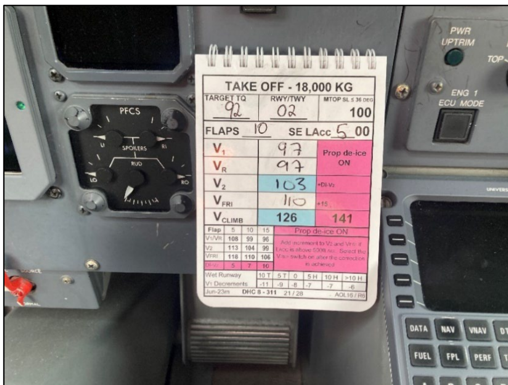
Figure 3: Take-off performance card (photographed after the occurrence)
