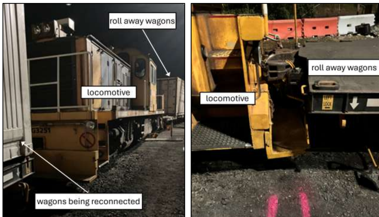
Figure 10: Position of locomotive and roll way wagons after collision
