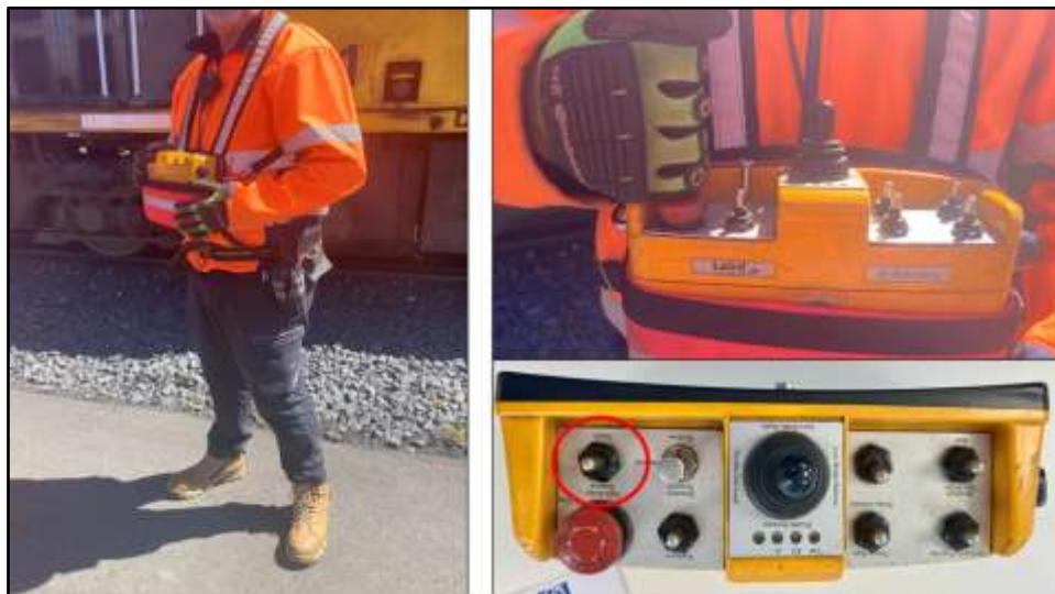
Figure 4: Remote-control pack as worn by an RCO
