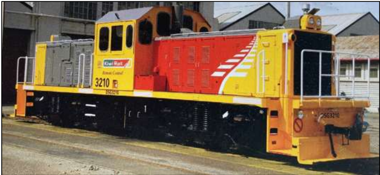
Figure 1: DSG-class remote-control shunt locomotive, similar to Y20 (Credit: New Zealand Railfan)
