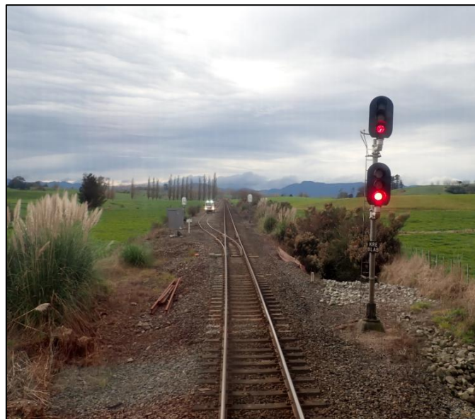
Figure 8: Entry signal (signal 8L) with the HVR in the Kereone crossing loop
