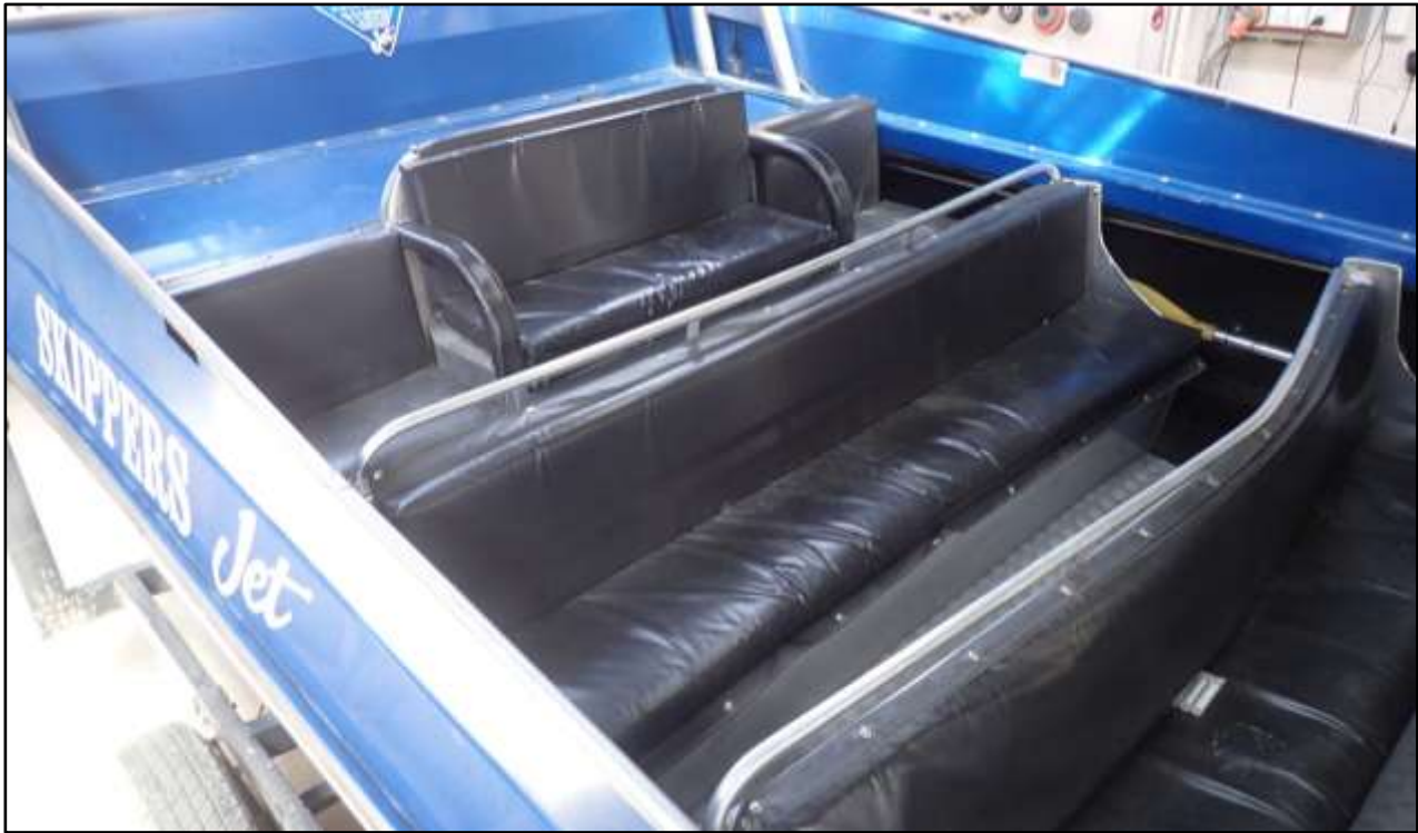
Figure 11: Deformation of seating and handrail from passenger's impact
