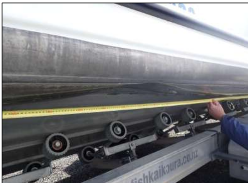
Figure 8: Indentation under port pontoon
