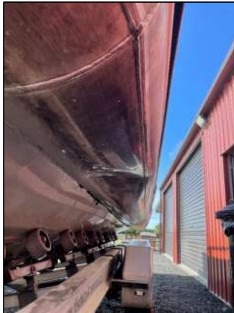
Figure 23: Indentation under port pontoon
