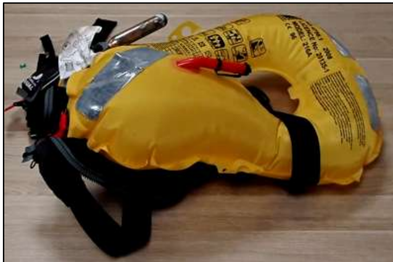
Figure 32: Bladder fully inflated after sudden violent burst of inflation
