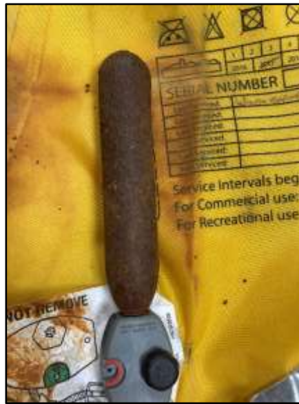
Figure 30: Corroded lifejacket cylinder
