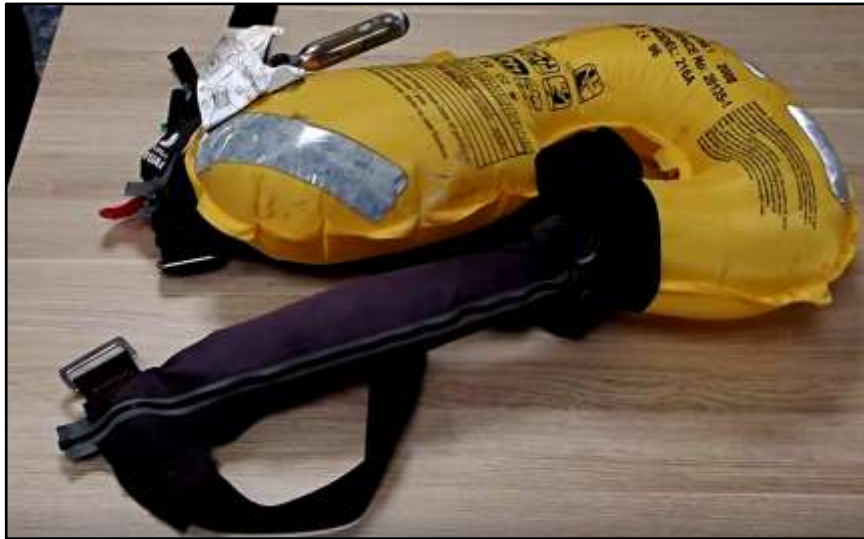
Figure 31: Lifejacket bladder pinched for several seconds
