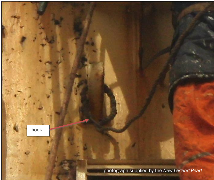
Figure 6 Safety harness lanyard hooked back onto itself
