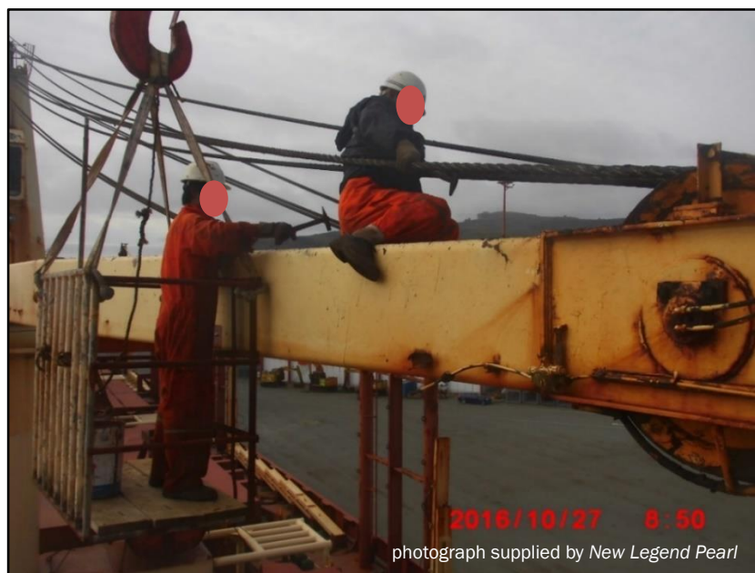
Figure 1 Crew working at height without full fall protection
