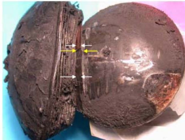
Scratches on the Stop (right) matched with the two laminations on the Laminated Portion (left). Yellow arrows indicate the gap in the two laminations due to the missing piece of top lamination.
