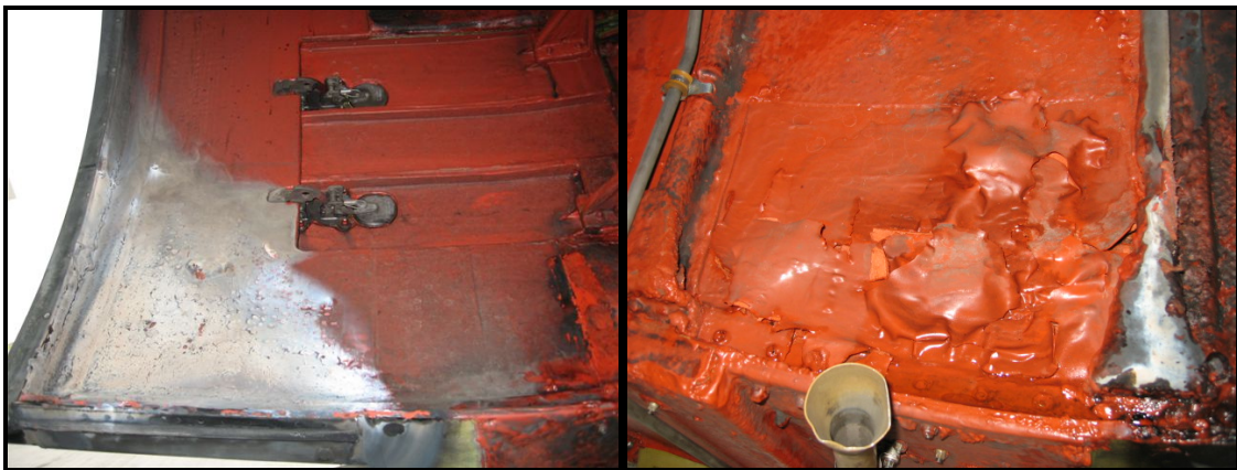
Figure 2 Damage to left engine cowls, ZK-NCK Left: thrust reverser inner diameter. Right: damage at 5-6 o’clock position.
