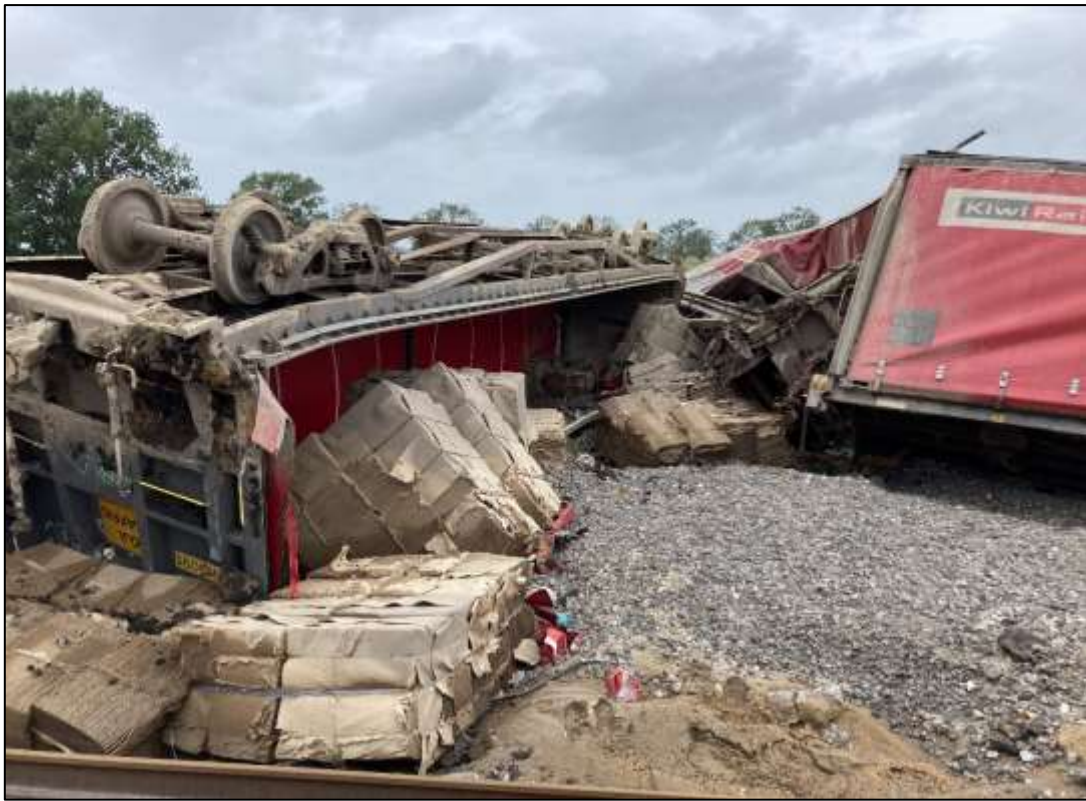
Figure 12: Derailed wagons and ballast debris on the eastern side of the rail corridor
