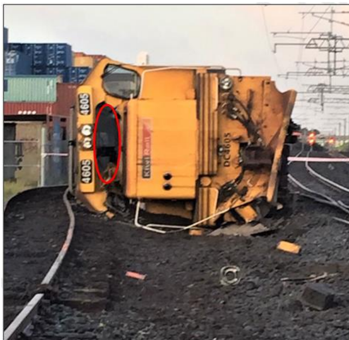
Figure 20: Locomotive following derailment, showing window through which crew exited.
