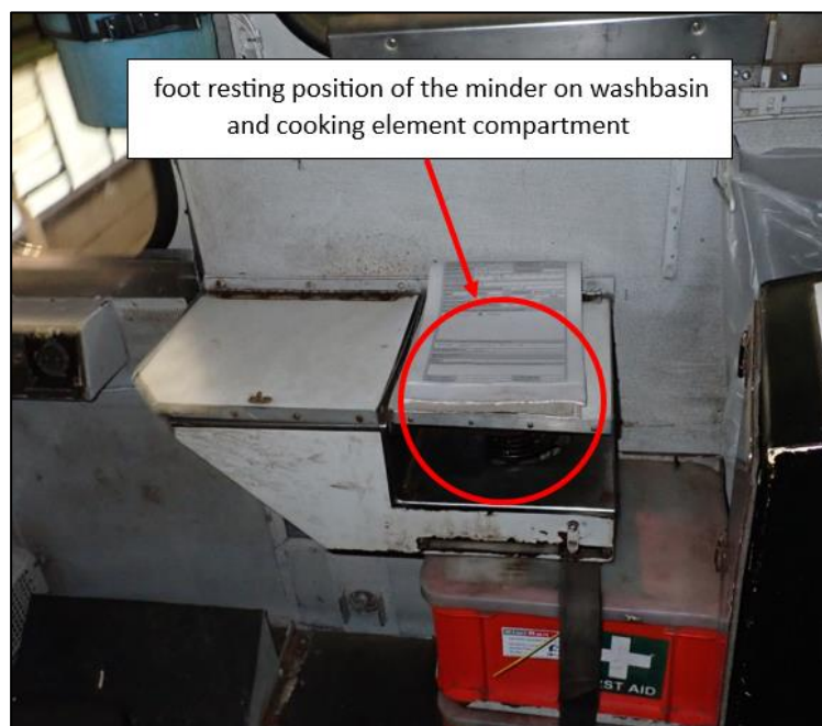
Figure 7: Wash basin on which minder rested their foot
