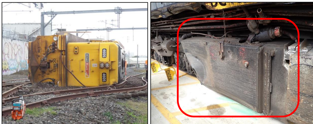
Figure 18: Position of locomotive following derailment (left) and ruptured fuel tank (right)
