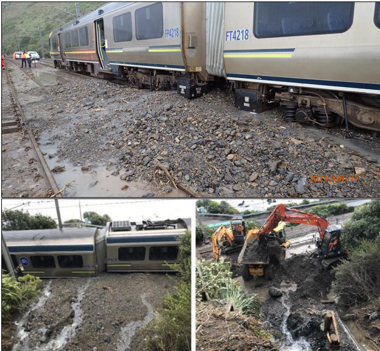
Figure 12: Rear portion of train with debris across the up and down main lines (Credit: KiwiRail).
