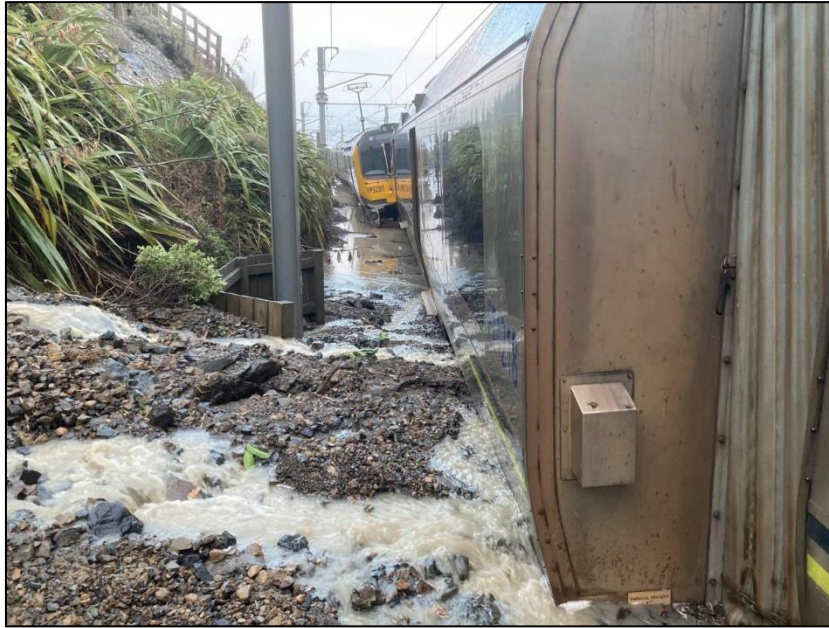
Figure 5: Derailed carriage and debris against and under carriage (Photographed at approximately 1210)
