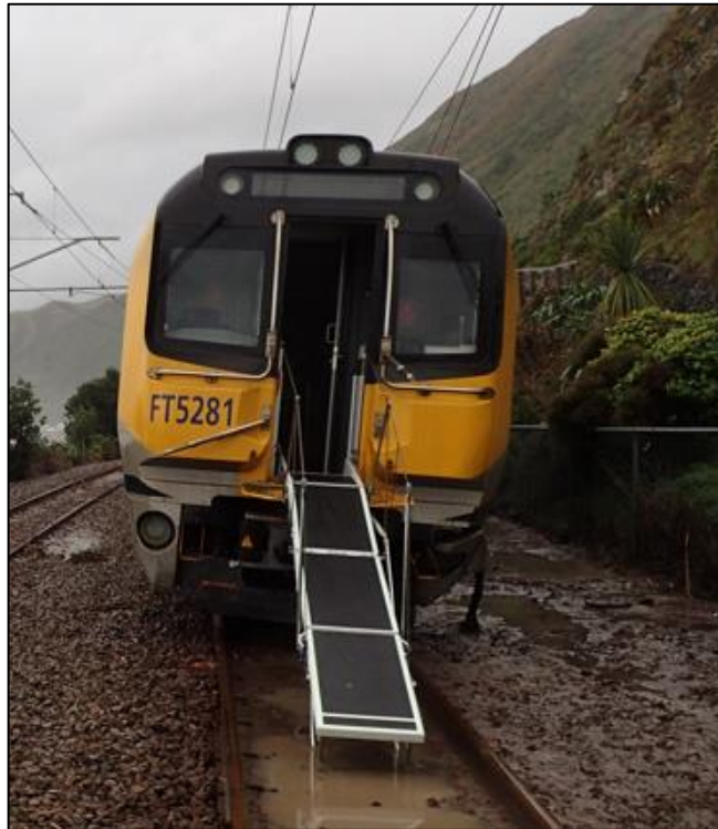
Figure 7: Passenger evacuation egress point from the train (Photographed at about 1215)
