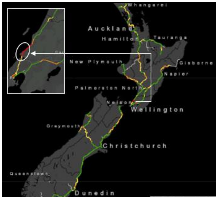
Figure 14: Rail resilience map showing the risk profile across the network (red – very high risk, amber – high risk, yellow – medium risk and green – low risk)
