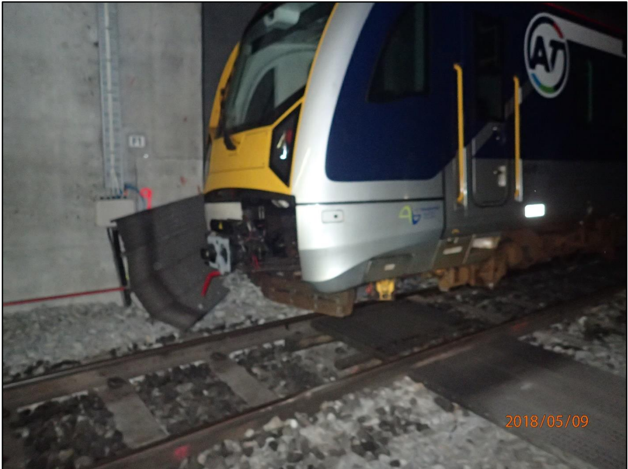
Figure 2 Derailed train stopped short of vertical dividing wall
