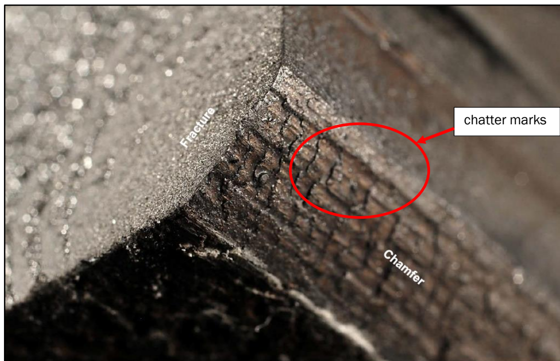
Figure 8 Origin of fracture at a chatter mark
