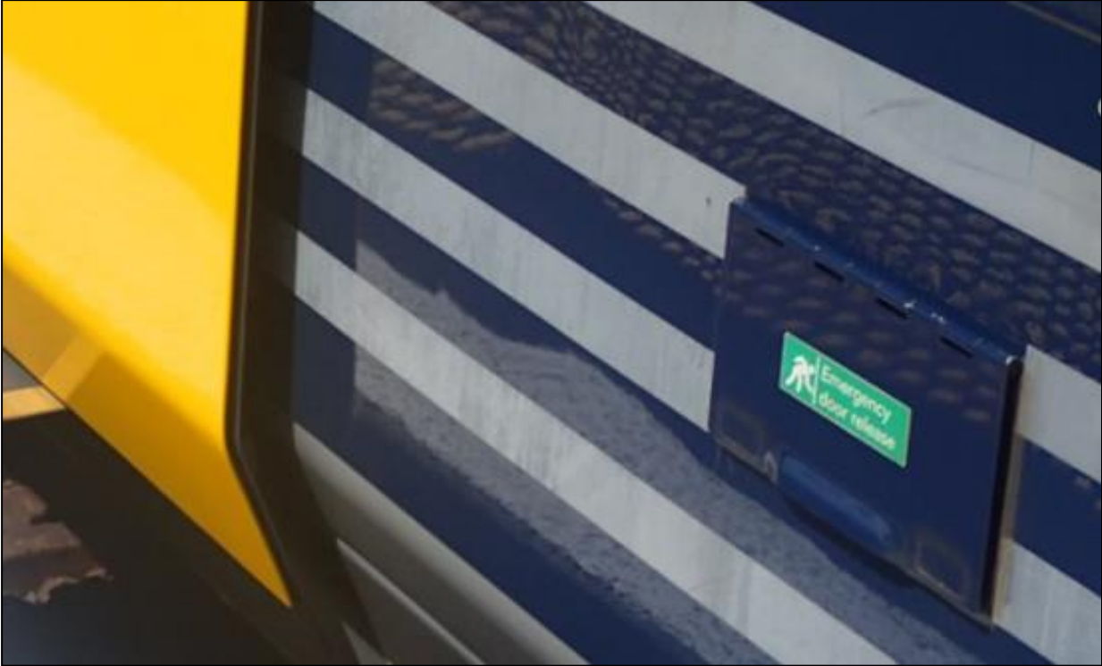
Figure 1 Covered emergency door release panel located on outside of passenger car
