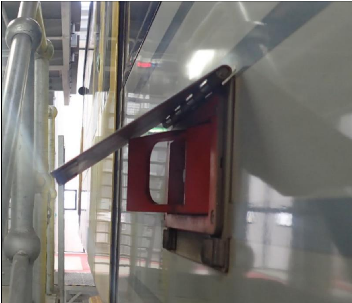
Figure 6 Emergency door release cover panel protruding from car
