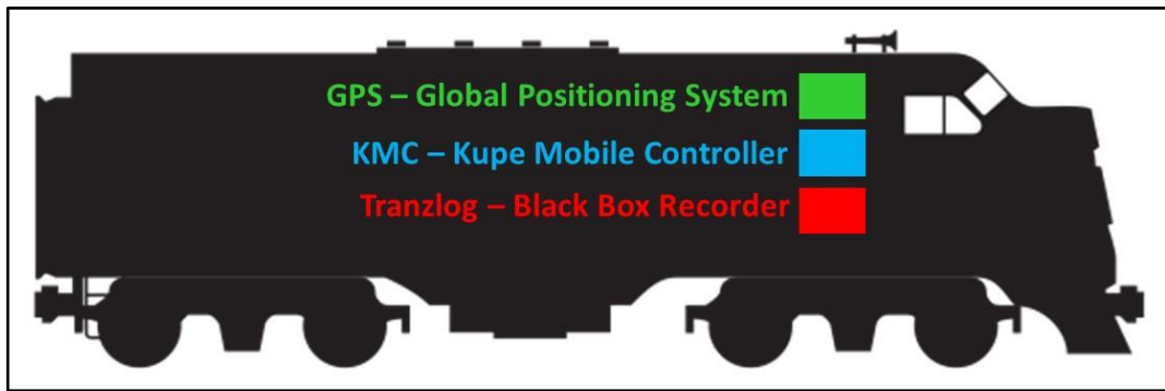
Figure 11 eProtect system component parts on board locomotives
