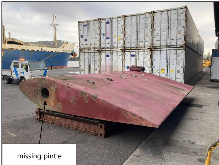
Figure 13: Bottom of rudder showing lower casting that previously housed the pintle
