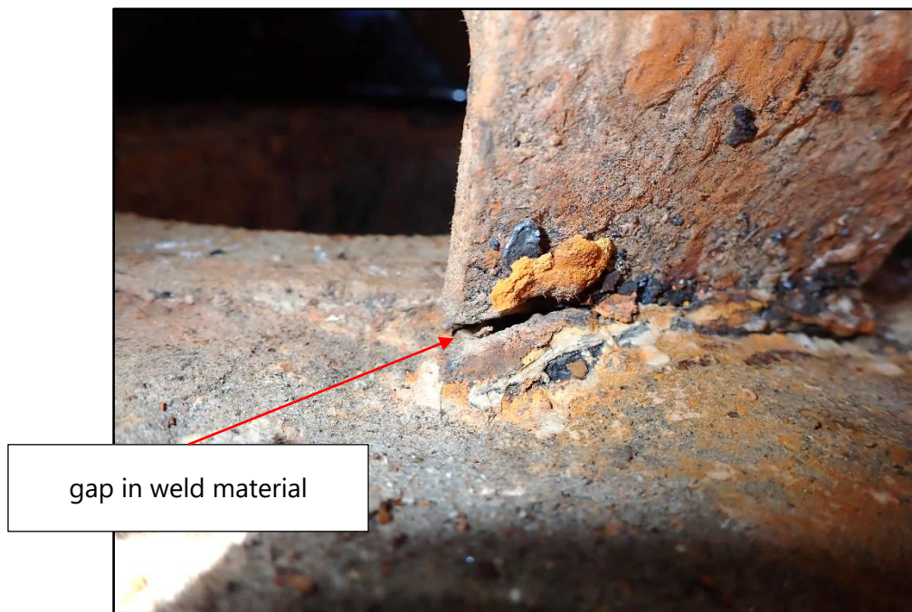
Figure 21: Weld connecting pintle stopper to interior of rudder blade
