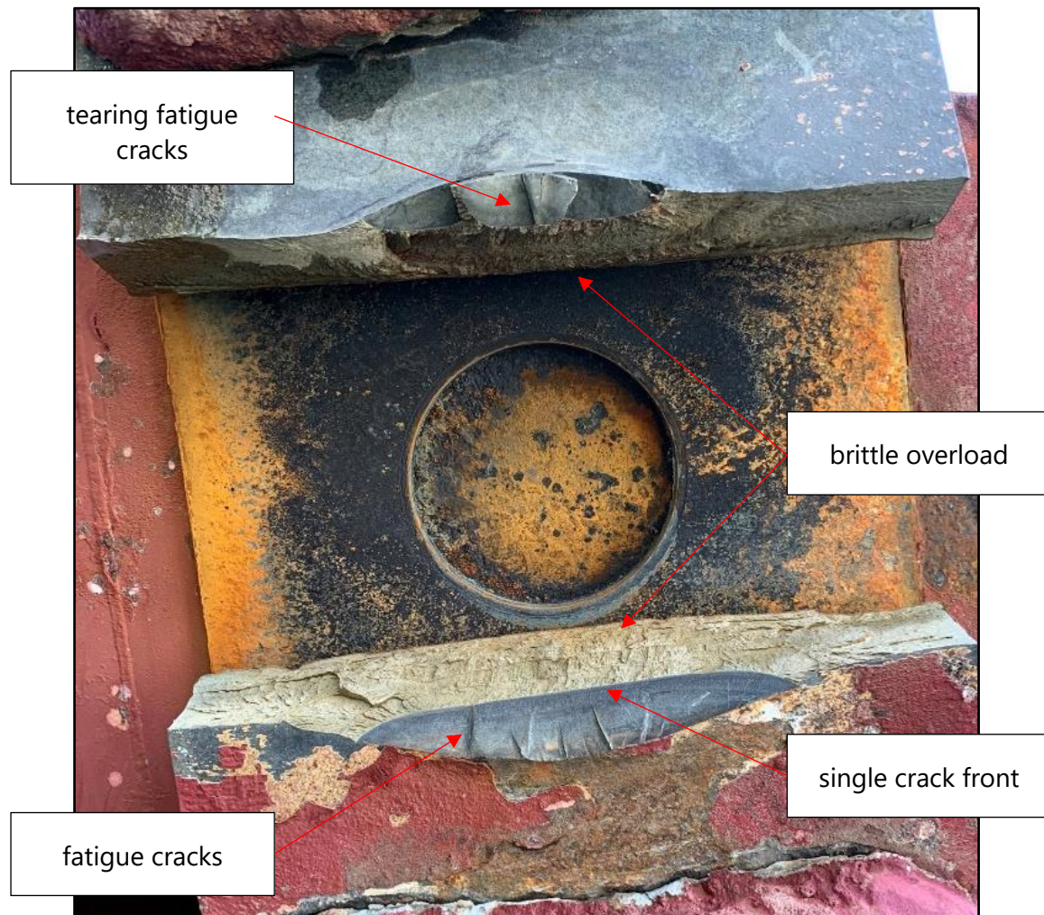
Figure 15: Fractured surfaces of rudder palm
