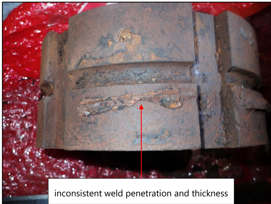
Figure 19: Weld connecting pintle stopper to side of nut 2021
