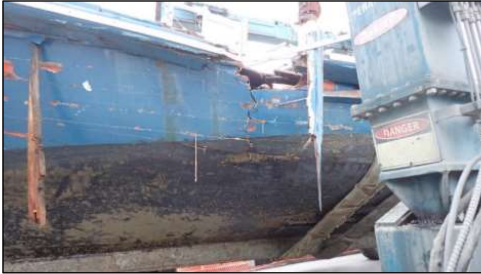
Figure 7: The Waitere hull damage as a result of the collision
