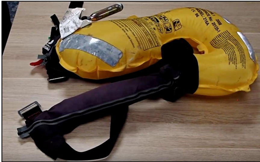
Figure 31: Lifejacket bladder pinched for several seconds
