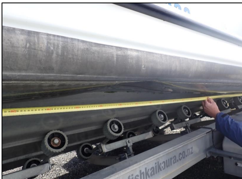
Figure 8: Indentation under port pontoon
