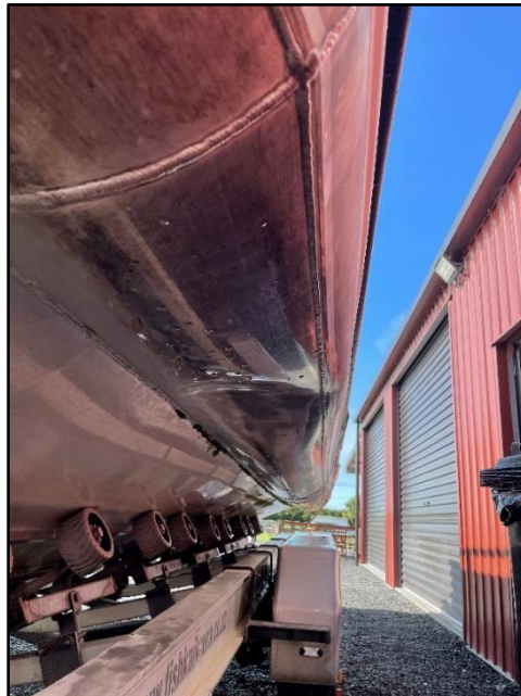
Figure 23: Indentation under port pontoon
