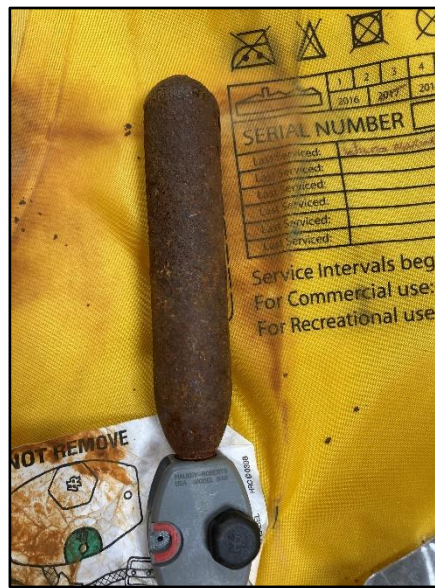
Figure 30: Corroded lifejacket cylinder
