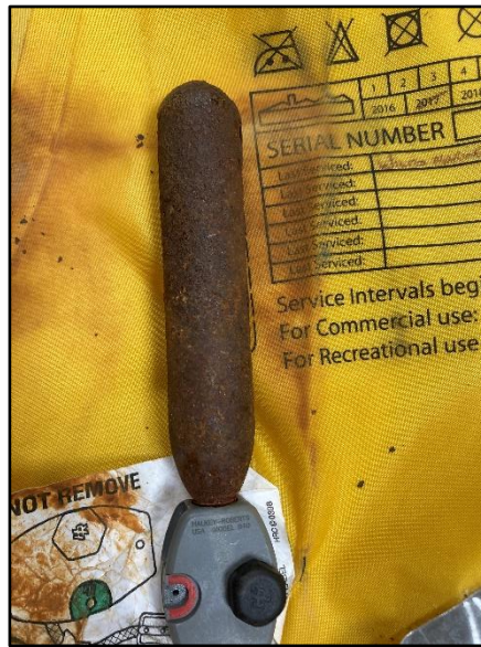
Figure 30: Corroded lifejacket cylinder
