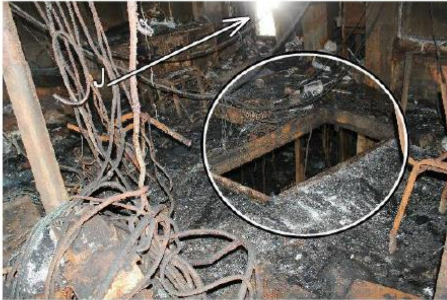
Photo 7: Looking across the bridge from the port side entrance the circle identifies where the ladder was that gave access to lower levels. 'J' shows the rear entrance on the starboard side.
