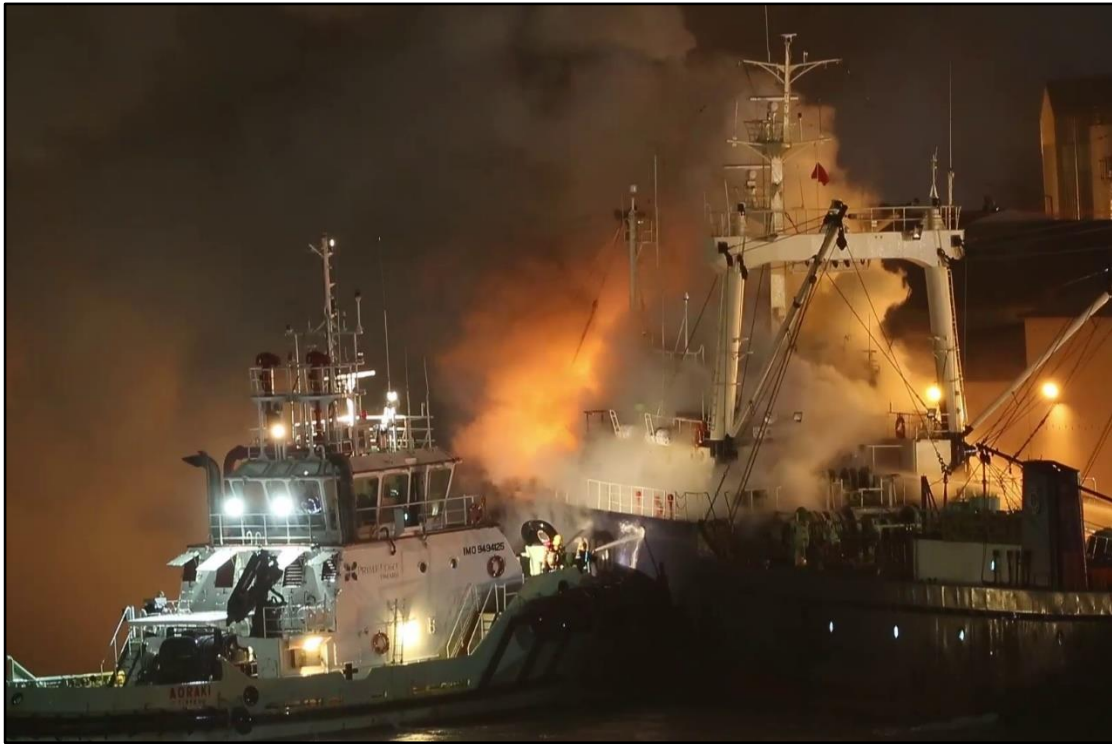
Figure 5: Tug Te Maru boundary cooling on the port side of the Dong Won 701
