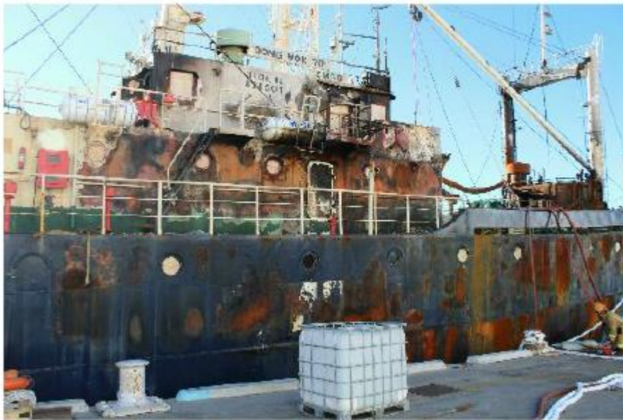
Photo 4: Shows the oxidisation on the superstructure and hull that is a result of excessive heat.
