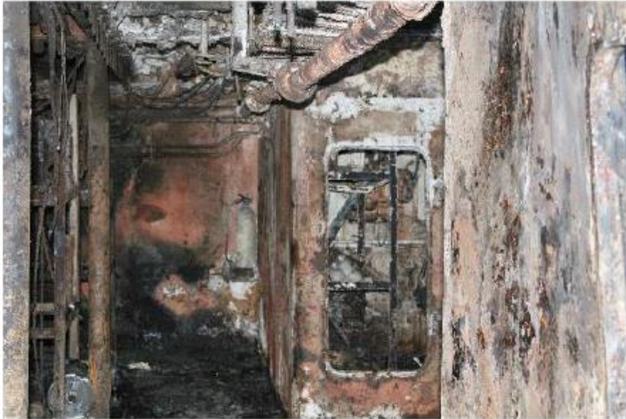
Photo 15: Shows the remaining paint on the walls of the Seamen's Living Quarters.
