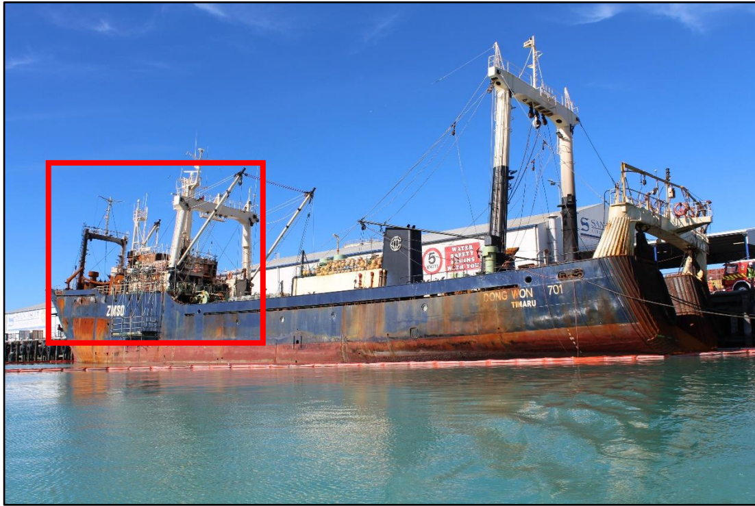
Figure 6: Area affected by fire marked in red
