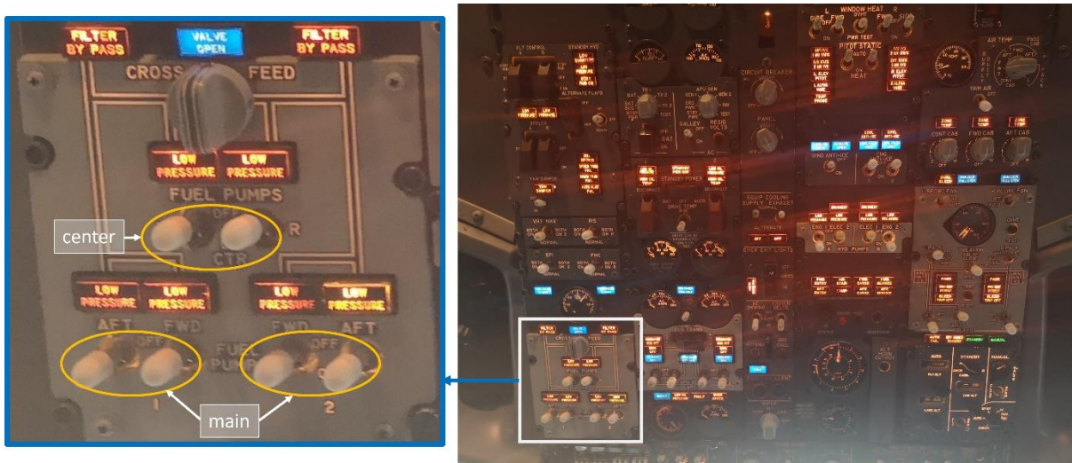
Figure 4: B737-400 overhead panel with fuel panel highlighted
