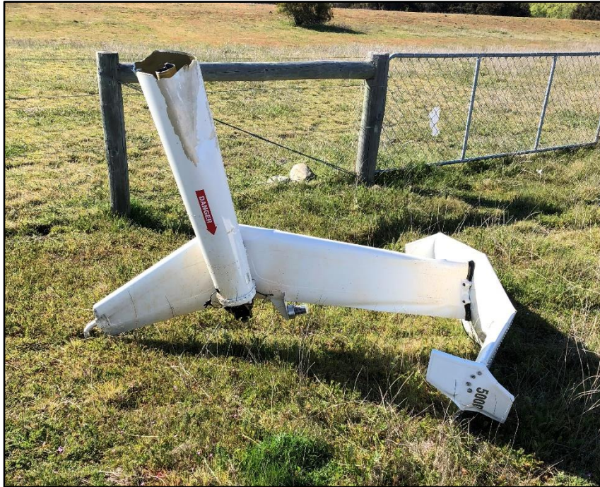
Figure 2 Photograph of separated tail section
