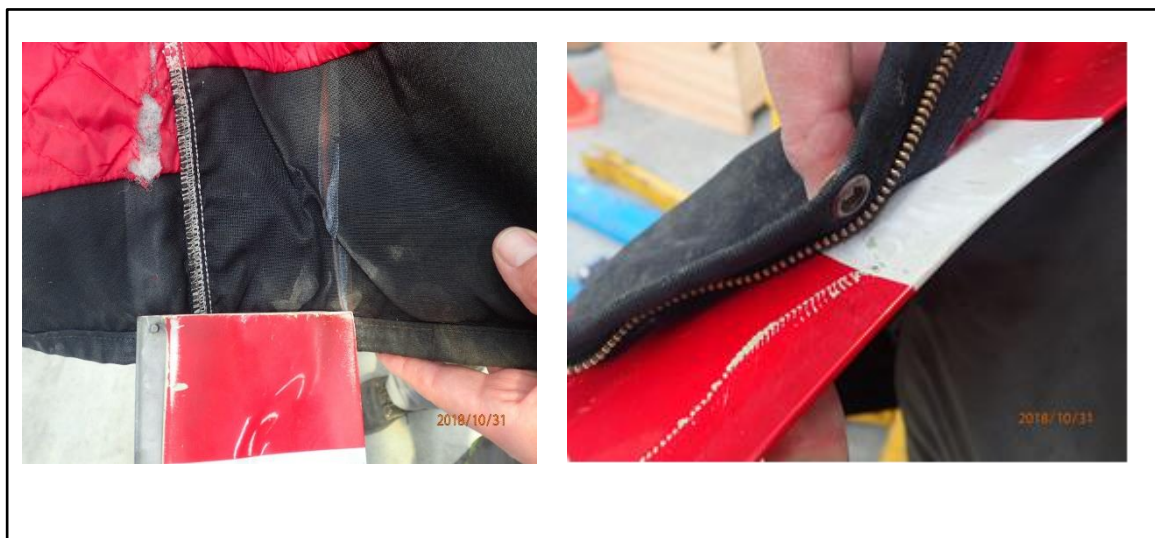
Figure 1 Tail rotor impact impressions
