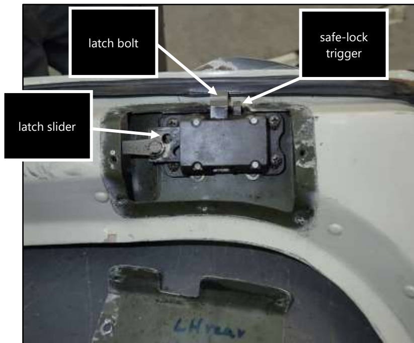
Figure 12: Latch block No.1 from left-hand rear door (cover removed)
