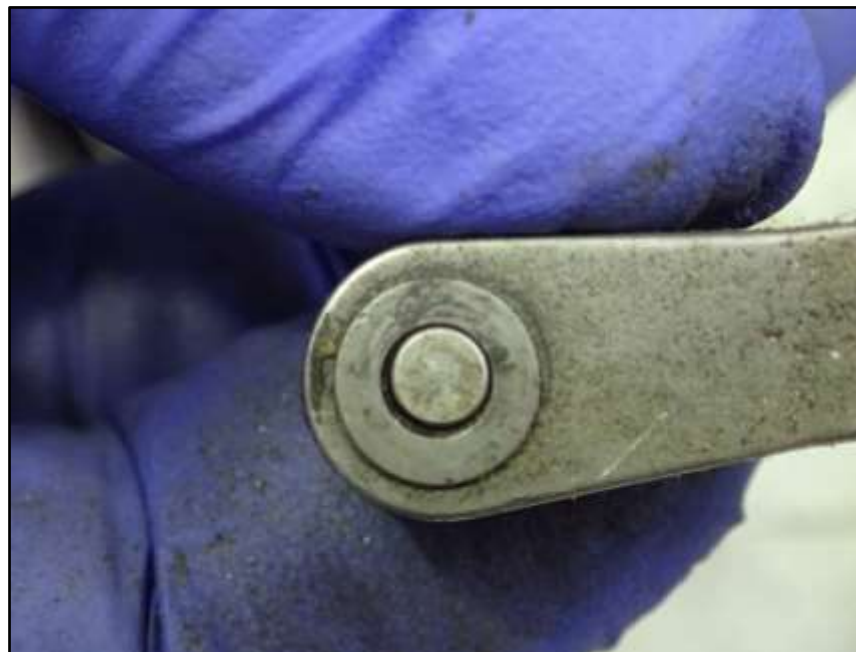
clevis and pin wear at top of latch block No.3 (door handle)
