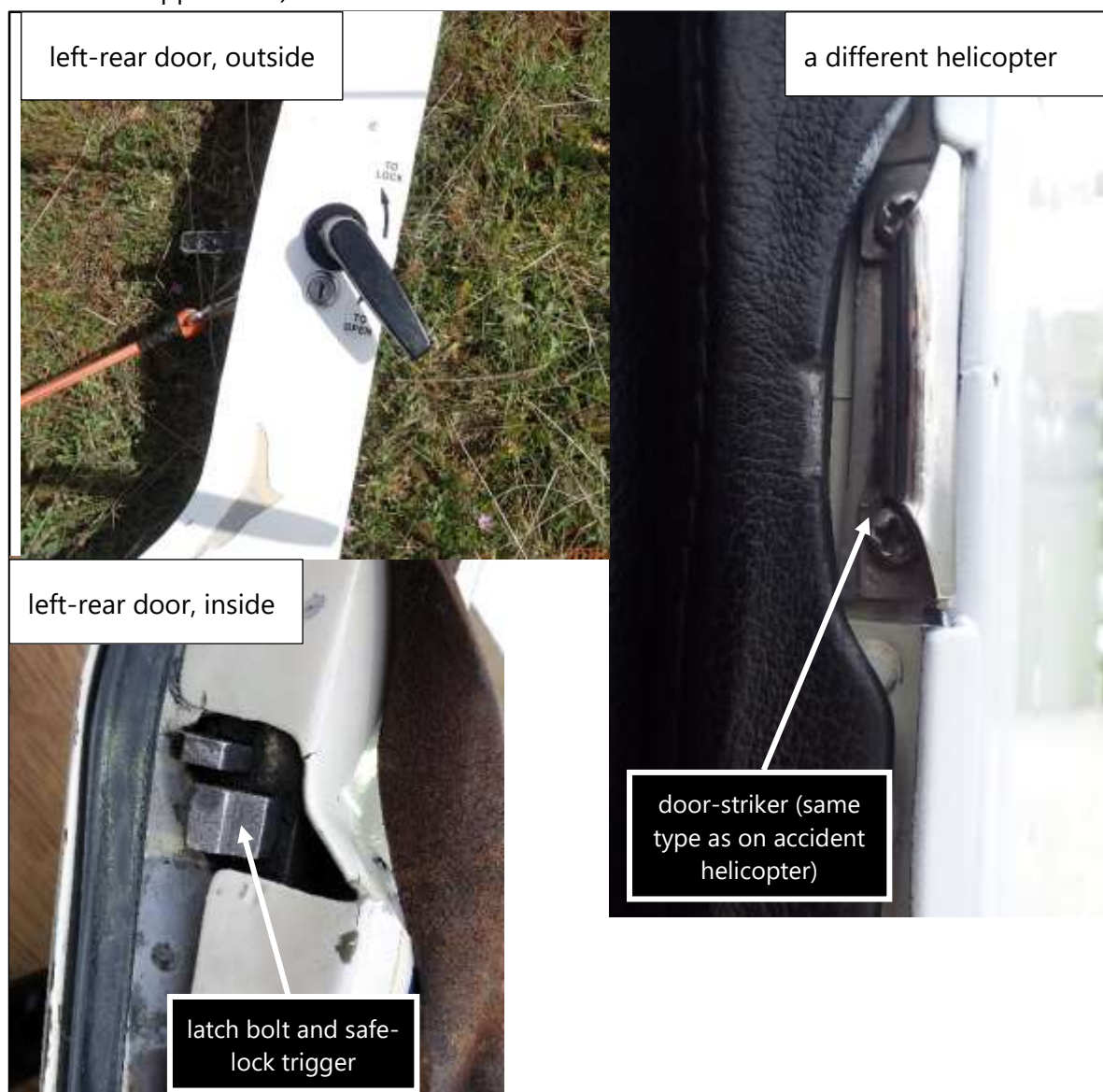
Figure 10: Rear door from the helicopter (left) and photograph of a door-striker on another helicopter (right)
