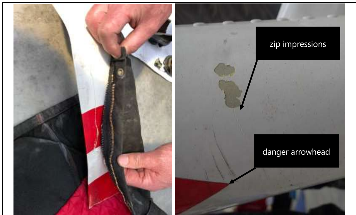
Figure 7: Black overalls' zip impact on tail rotor blade and tail boom
