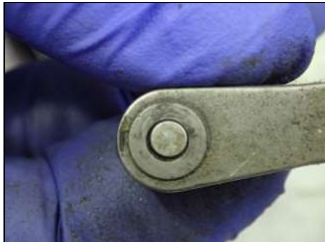
Figure 14: Clevis pin wear
