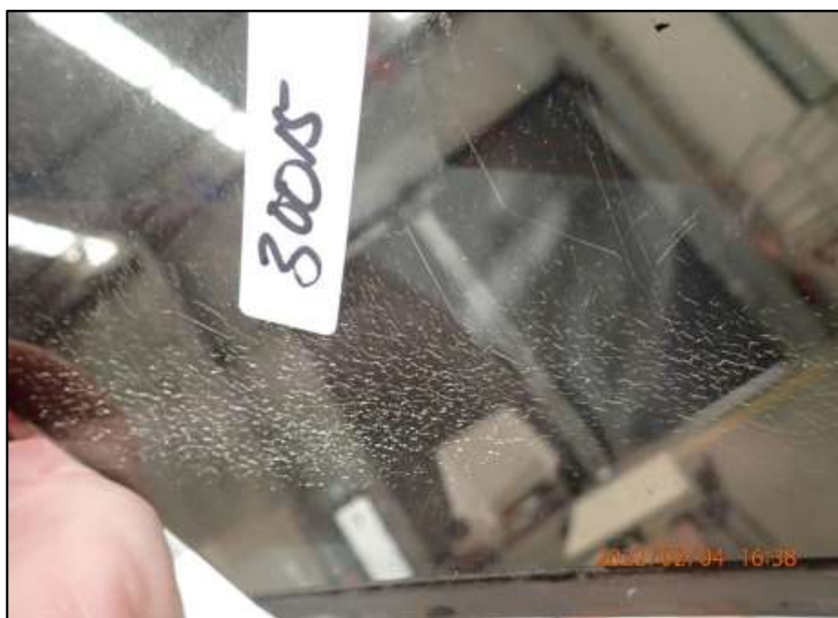
Figure 17: Crazing in centre-right windshield
