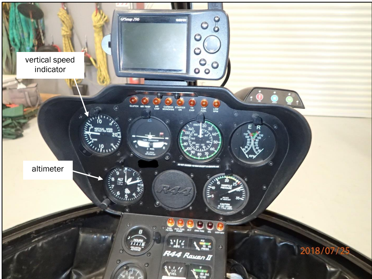
Figure 3 Typical R44 flight instrument panel
