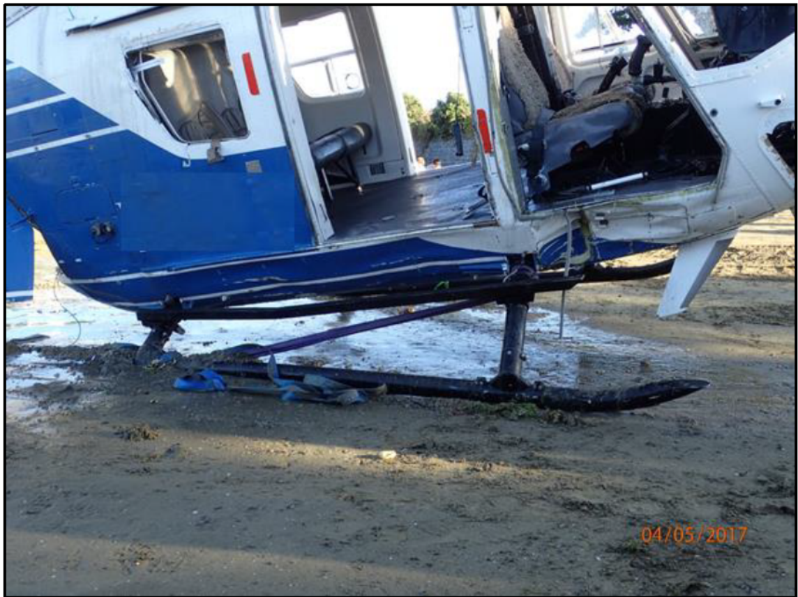
Figure 4: Hydrodynamic damage to fuselage
