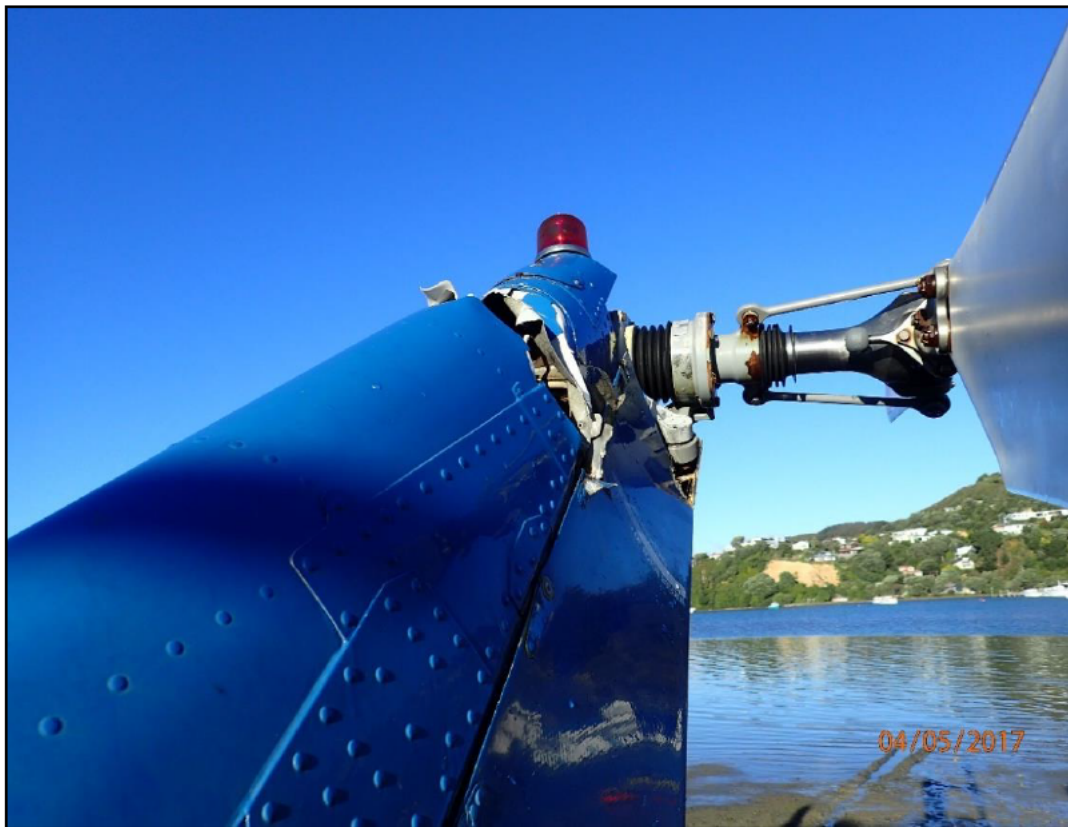
Figure 5: Failure of vertical fin
