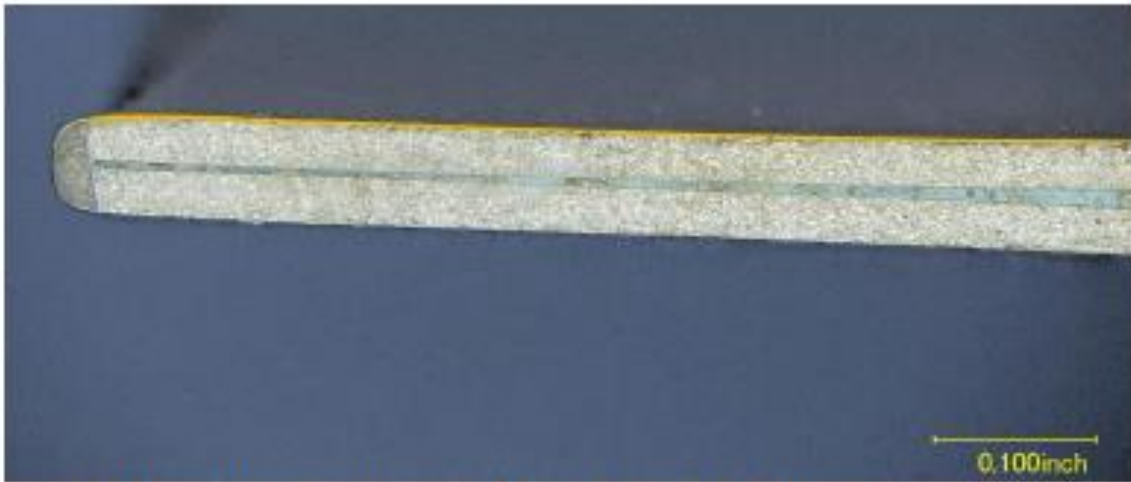
Figure 6 – The initiation point of the fatigue crack at the trailing edge of the main rotor blade.
