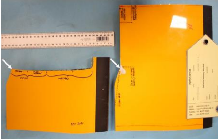
Figure 1: Fractured blade sample shown at left, matching location on opposite blade shown at left. Trailing edge transition radius arrowed on both samples. Upper surface shown
