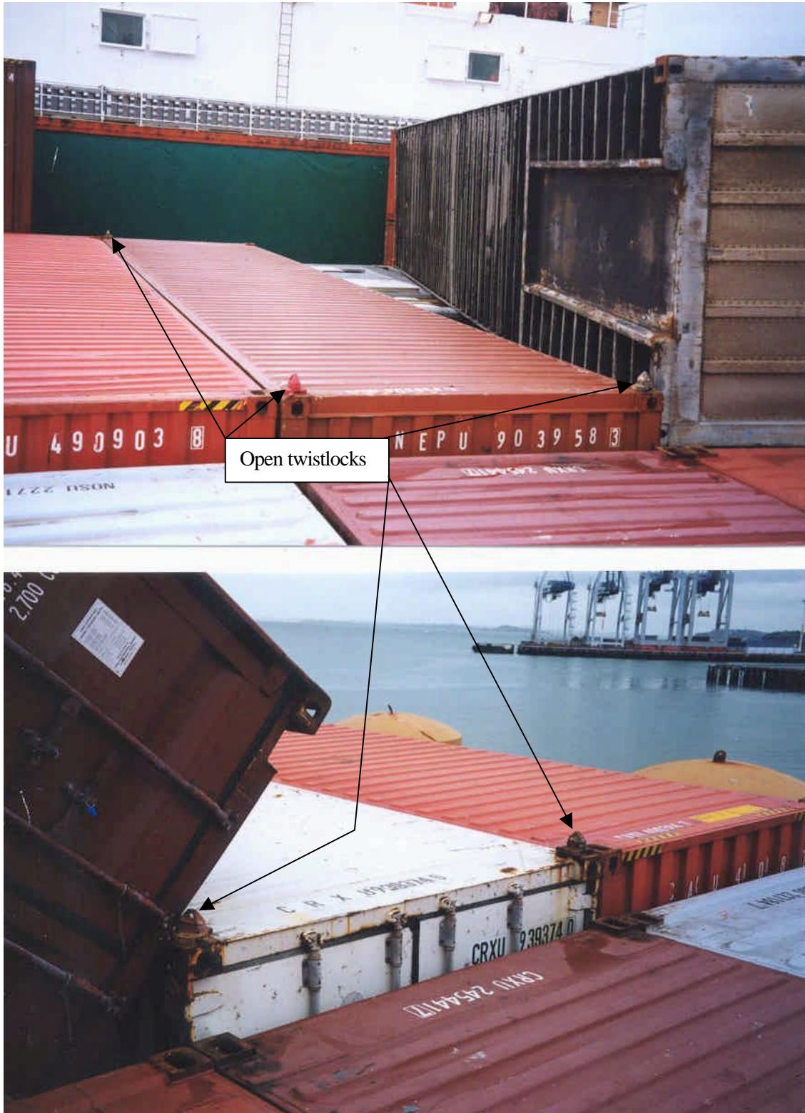
Figure 9 Photographs showing toppled containers on upper deck (note open twistlocks)
