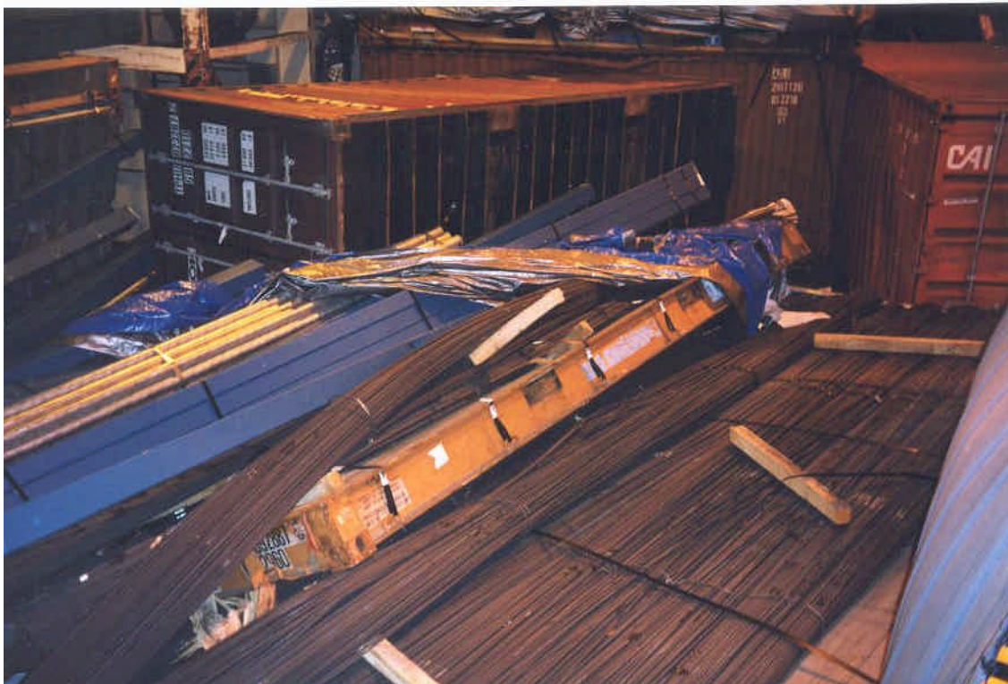
Figure 10 Photographs of cargo damage in the main vehicle deck
