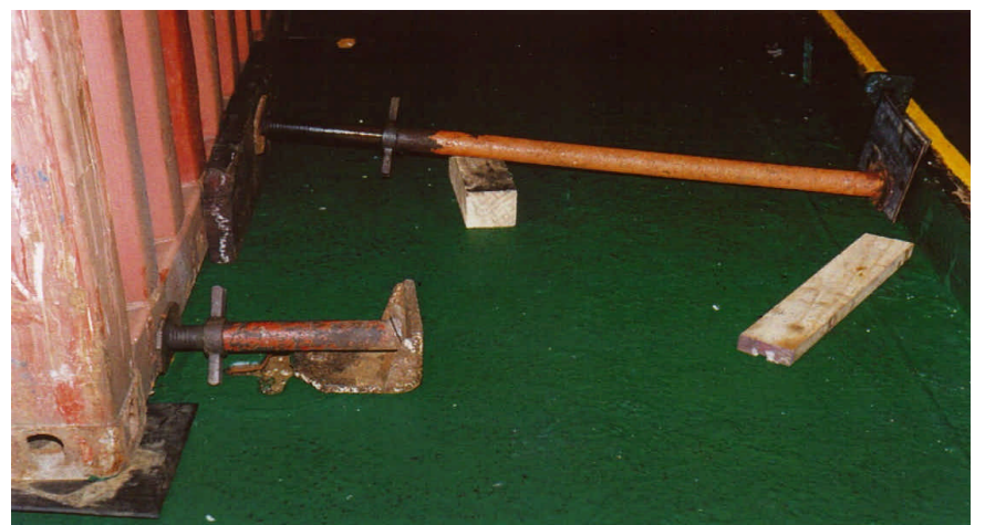
Figure 8 Photographs of lashing equipment used in main vehicle deck and lower hold, copied from cargo securing manual
