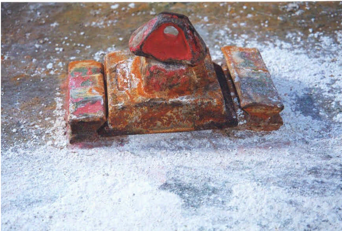
Figure 11 Photographs of worn deck sockets and twistlocks
