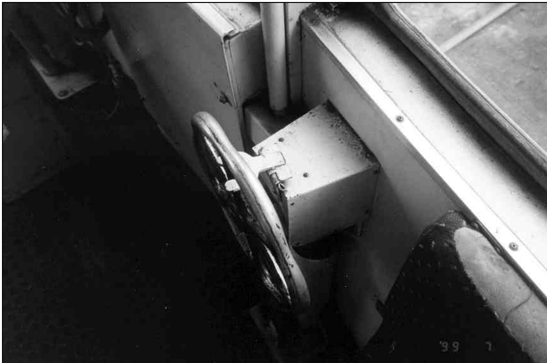
Figure 5 A handbrake with restraining clip at the top, but with no locking facility
