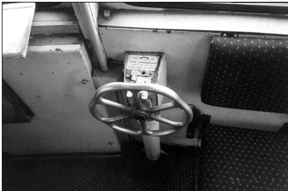
Figure 3 The handbrake in an ADB car showing clip in place and square key lock
