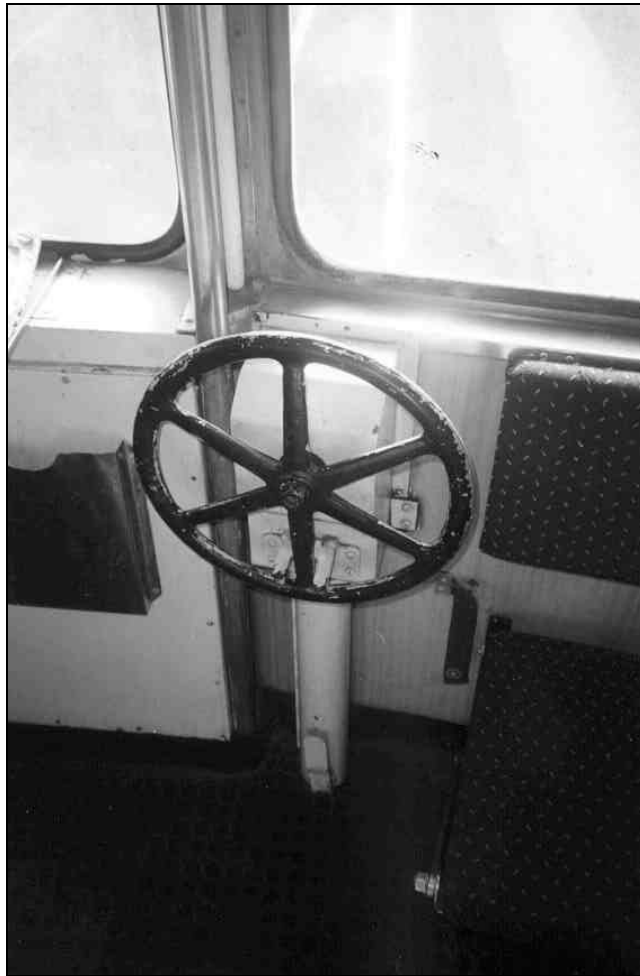
Figure 2 A typical handbrake with restraining clip at the bottom, but with no locking facility, as used on ADKs
