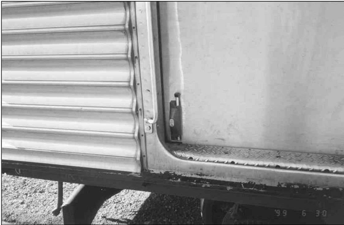
Figure 4 A lockable outside bolt on a driving cab external door
