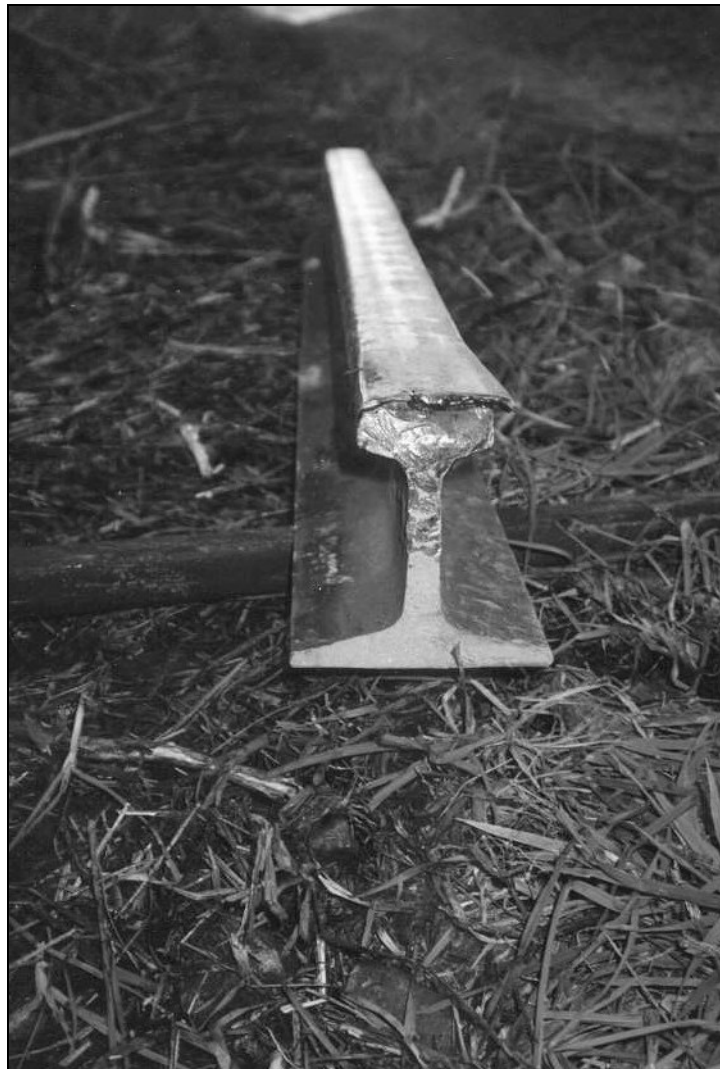
Figure 2 End view of the original failure face (north side of break)
