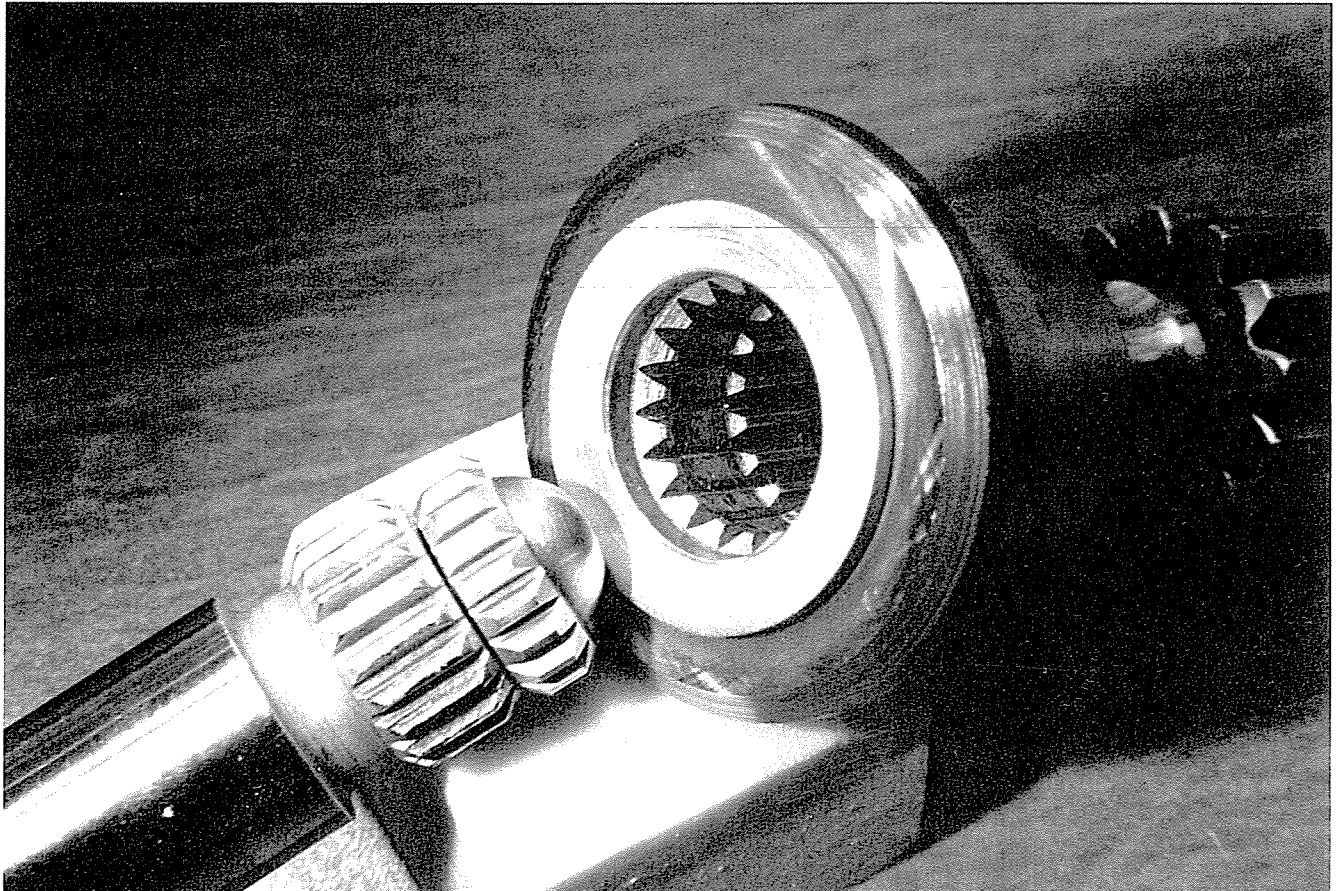
2. Fuel Pump Drive Shaft internal spline wear, wear on loaded side of driver gear teeth and circumferential scoring.
