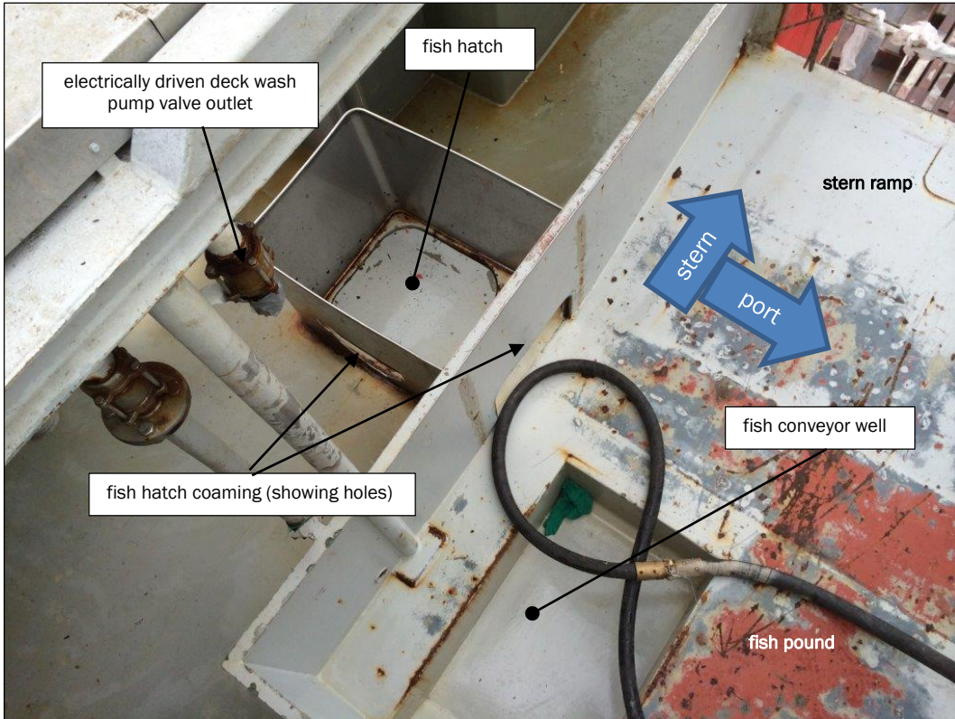
Figure 9 Fish pound and fish hatch on the Jubilee (photograph taken in dry-dock, from above)
