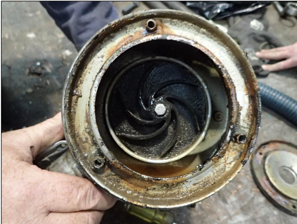
Figure 11 Shore-based examination of the recovered electric bilge pump from the fish hold
