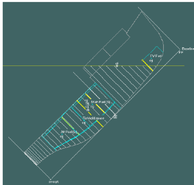
Fish hold 75% flooded; with 75% fuel in aft tanks (forward section down-flooding?)
