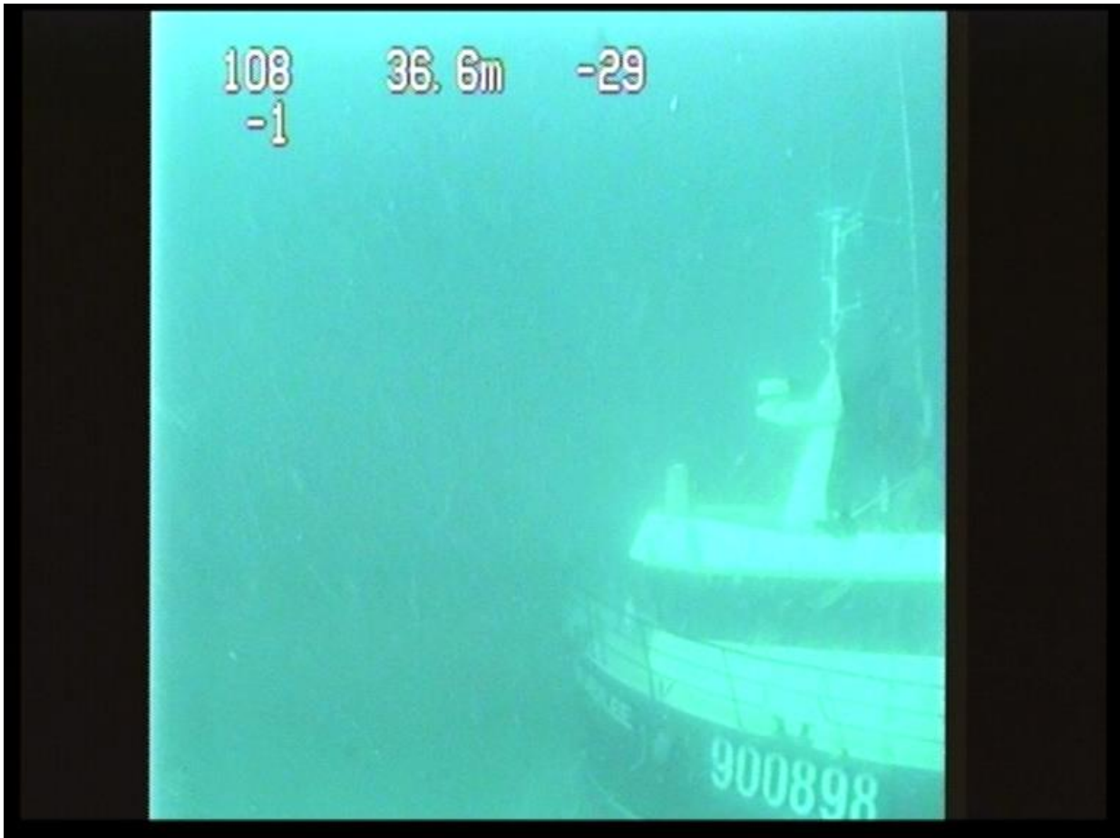
Figure 4 Video still from the remotely operated vehicle search for the Jubilee , showing the vessel sitting upright on the seabed
