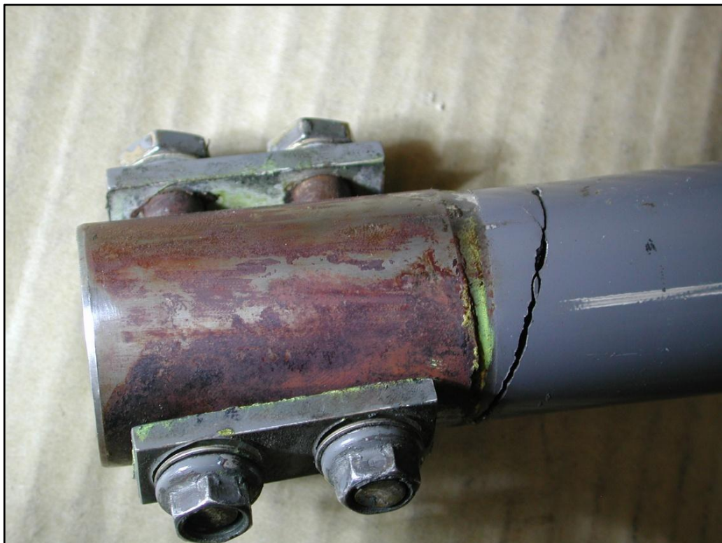
Figure 7 Cracked clutch shaft
