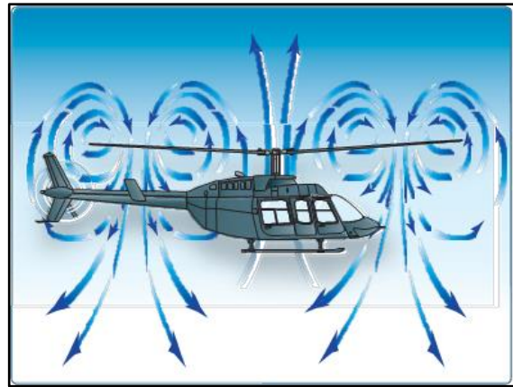
Figure 8 Vortex ring state (Courtesy of Federal Aviation Administration)
