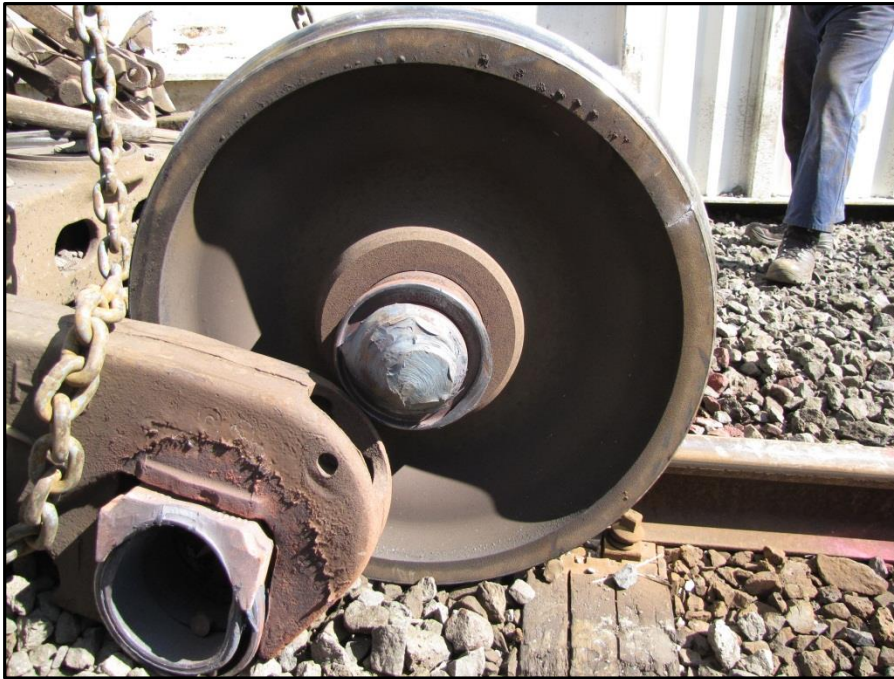
Figure 4 “Screwed” axle journal from the derailed wagon
