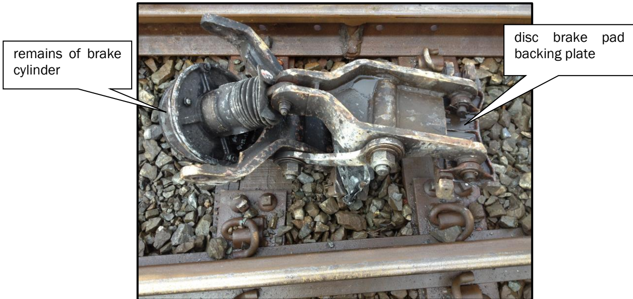
Figure 3 Spring park brake mounting bracket with part of the brake cylinder
