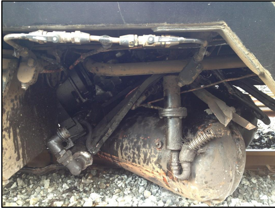
Figure 4 Air reservoirs jammed under air compressor
