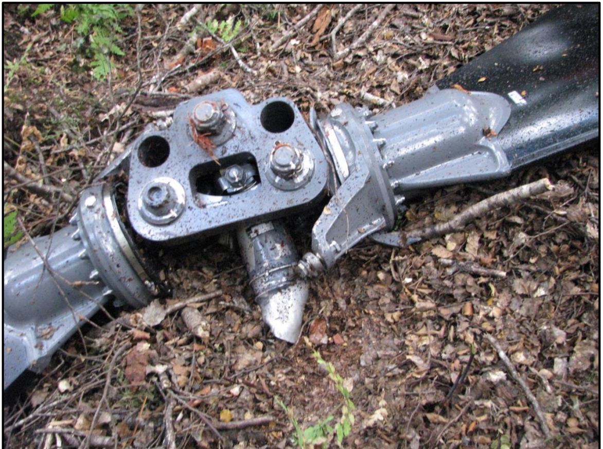
Figure 3 Main rotor head, showing severed drive shaft
