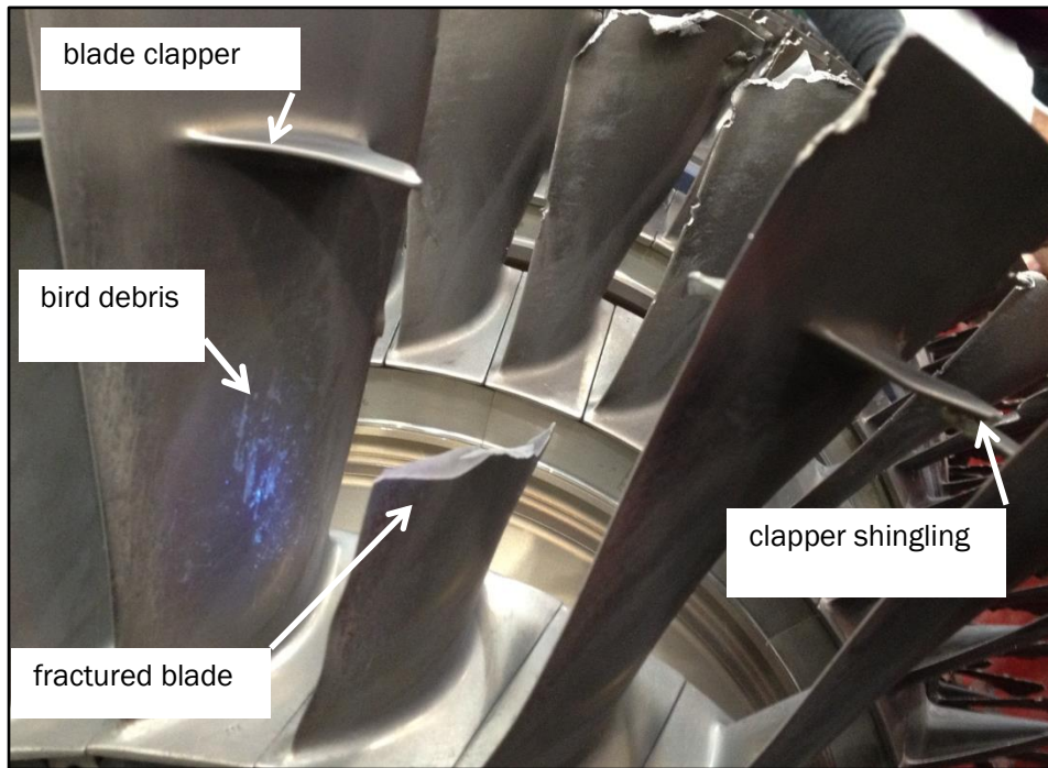
Figure 1 Fractured third-stage blade and an example of clapper shingling
