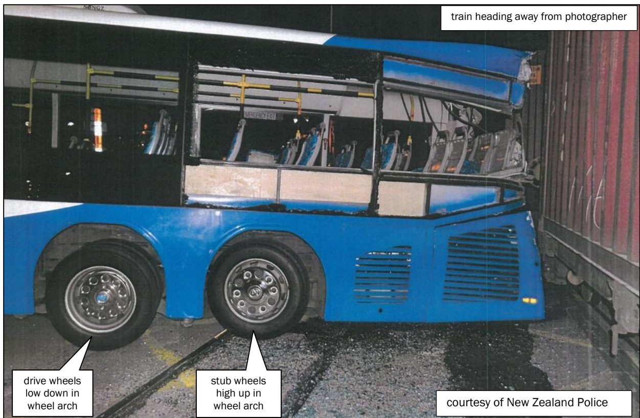
Figure 1 Photograph of the collision aftermath (looking south)
