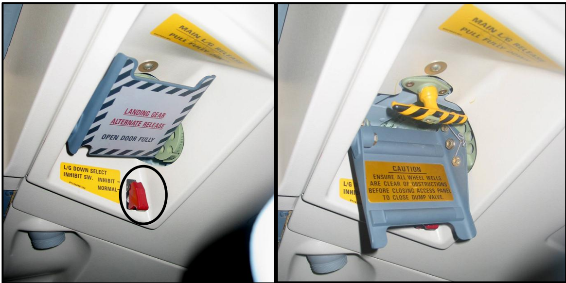
Figure 1 Landing gear alternate release door (above first officer's seat), with inhibit switch circled (Photograph courtesy Air Nelson Limited)
