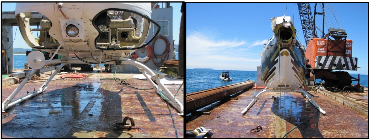
Figure 3 Fuselage underside, after recovery
