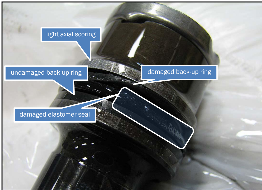
Figure 7 Nose landing gear actuator piston removed from ZK-NEB
