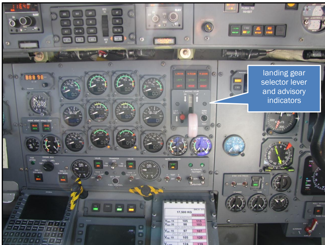
Figure 1 Q300 flight deck, centre instrument panel
