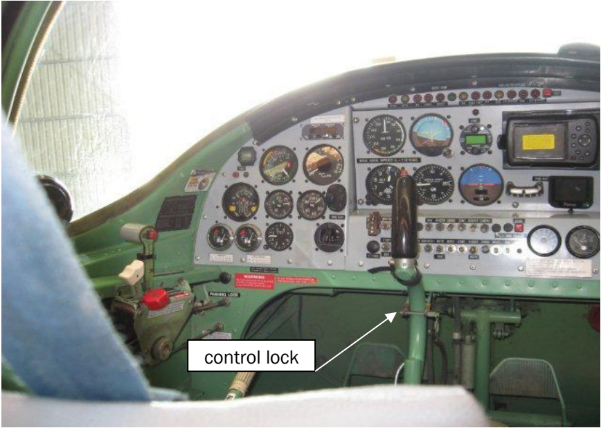
Figure 5 Control lock (Courtesy of M Feeney)
