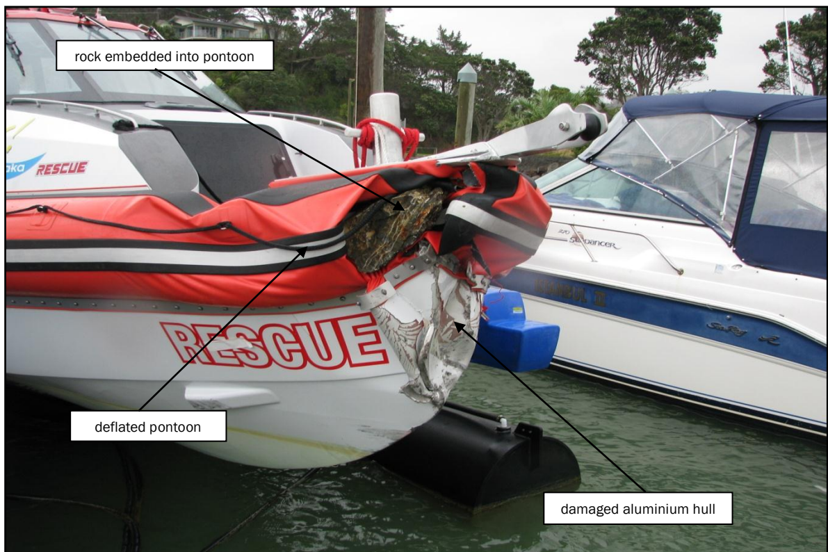
Figure 7 Bow damage to the Dive Tutukaka Rescue
