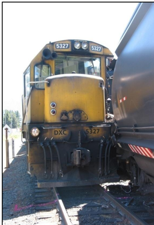
Figure 7 Lead locomotive of Train 848 wedged against Train 845
