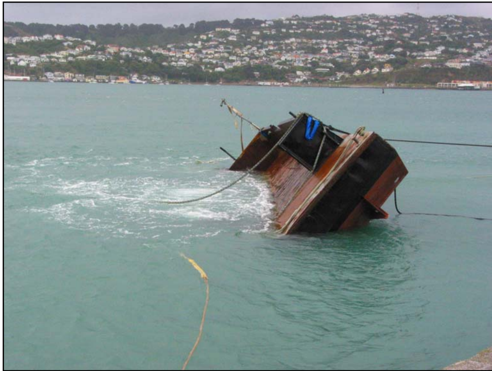
Figure 8 The Kimihia in the process of being righted
